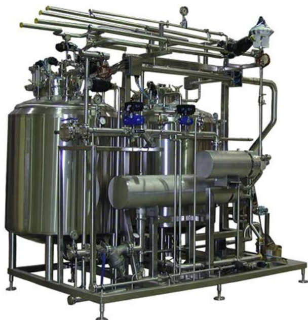
FIGURE 26.29 A typical clean-in-place system used to clean upstream and downstream process equipment. The tanks in the background are used to mix and heat up the cleaning solutions before delivery of the cleaning solutions to the downstream process equipment through a network of piping. (Source: Turn-Key Modular Systems. http://www.tkmodular.com/StandardProducts/CIPSystems.aspx .)
