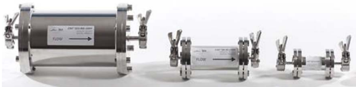
FIGURE 26.27 A membrane chromatography column. The steel cylinder contains a 3-D matrix with bound ligands rather than spherical beads. (Family of CIM® Monolithic Columns from BIA Separations.) (Source: BIA Separations. http://www.biaseparations.com .)
