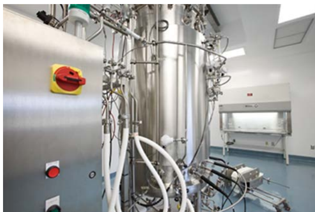
FIGURE 26.18 Mammalian upstream bioreactor operations. (Source: Cytovance Biologics Inc., 2013.)
