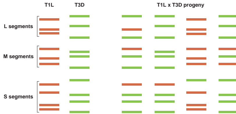
Figure 19.2 Generation of reassortant viruses. Reovirus strains are distinguishable by unique electrophoretic profiles of their double-stranded RNA gene segments. Coinfection of cells with different viral strains produces a collection of progeny reassortant viruses containing various combinations of gene segments from each parent. Shown here are schematized diagrams of electrophoretic profiles of prototype strains type 1 Lang (T1L) and type 3 Dearing (T3D) along with some reassortant progeny.
