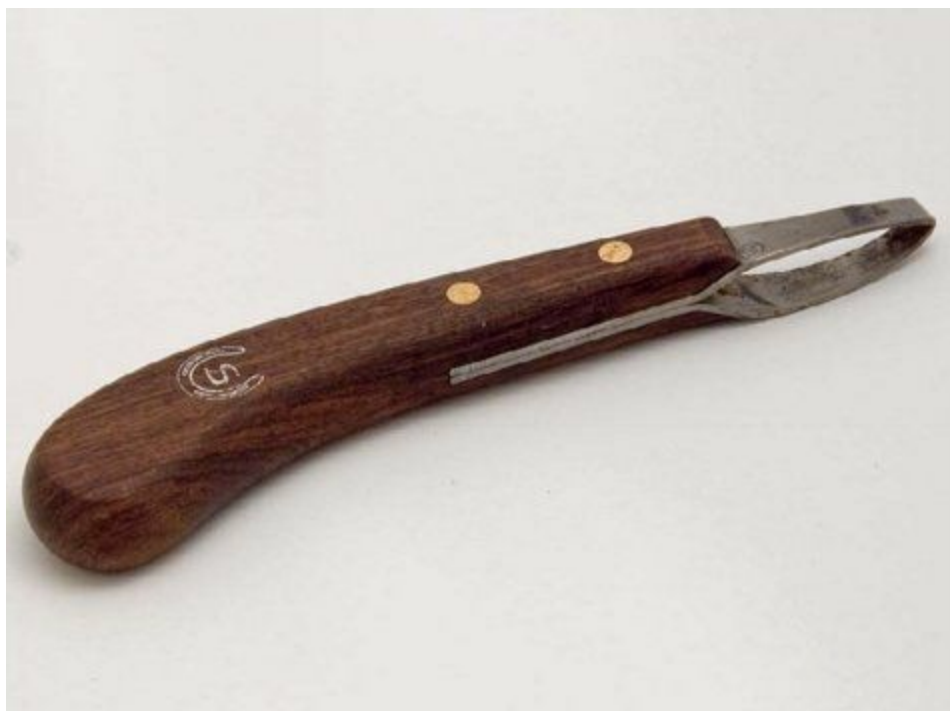
Fig. 1.9. Loop knife. © O.Grishko
