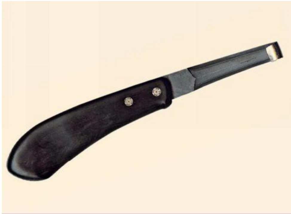
Fig. 1.8. Double-sided hoof knife. © Nevzorov Haute École
