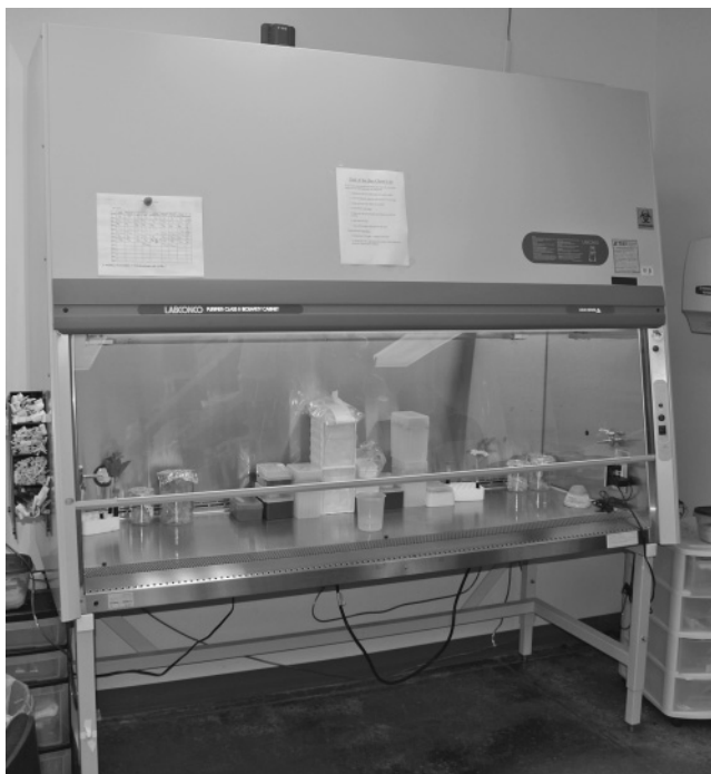
Figure 5.1 Class IIA, vertical laminar flow biological safety cabinet. Although this cabinet is very long, much shorter cabinets are made, which can easily fit into smaller spaces.
