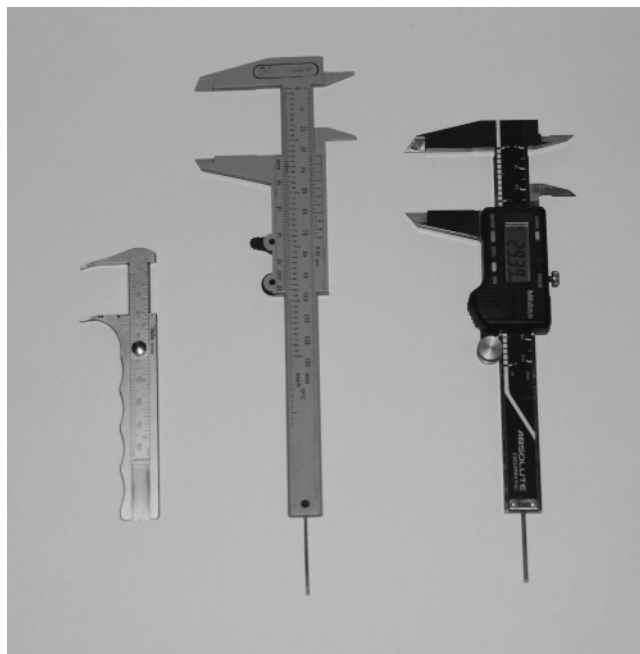
Figure 4.3 Different styles of calipers. Calipers can be purchased at most hardware stores, as well as from veterinary or surgical supply vendors.
