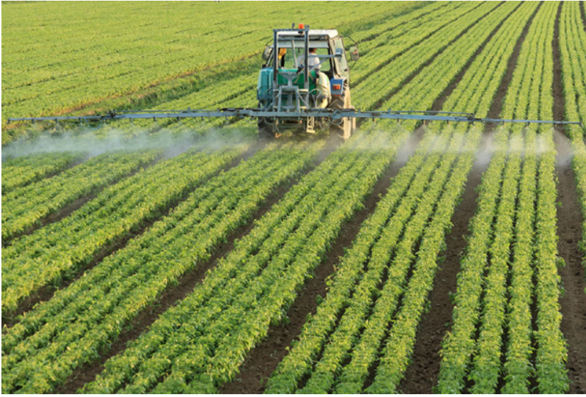
FIGURE 6.1 Spray application of insecticides to row crops. Applicators are much better protected inside a tractor with a cab, especially if the windows are shut and the cabin filtration system is properly functioning. (Source: Frederico Rostango/Shutterstock.com.)
