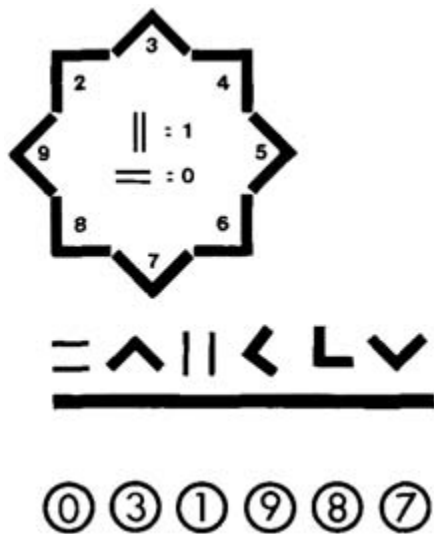
Fig. A2.2. The angle code for freeze marking. The orientation of the angle or parallel bars represents an integer (above), as shown in example (below). (Adapted from Farrell and Johnston 1973.)
