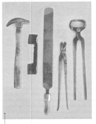
Left to right: Hammer, Clinch Cutter, Rasp, Crease Nail Puller, Pull-off
