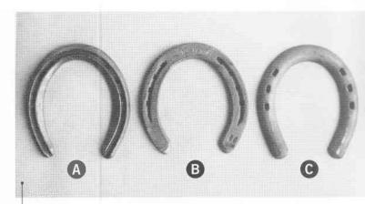
Three Types of Horseshoe Ground Surfaces A rim shoe (A) has a deep crease down the center of the entire ground surface that forms two rims for added traction. A plain horseshoe (B) has a crease on each branch extending slightly past the first and last nail holes. A stamped shoe (C) has no crease; instead, the nail holes are enlarged at the top to recess the nail heads.
