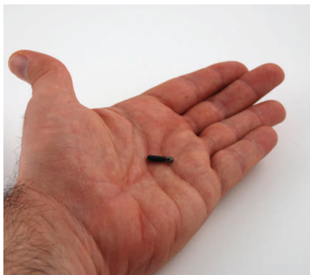
FIGURE 16–8 Size of an RFID tag in comparison to the human hand.
