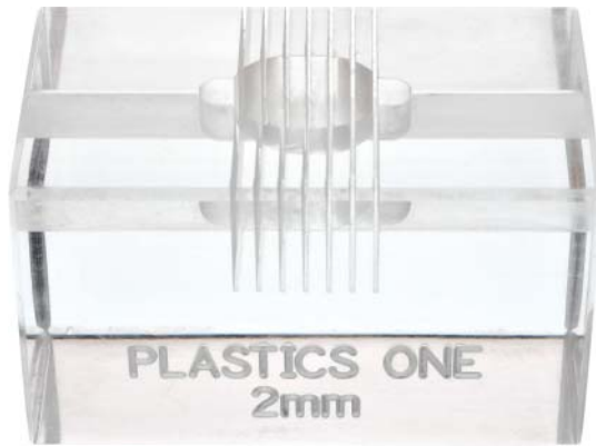
Figure 8.6 Brain matrix to aid reproducible cutting of brain slices.
