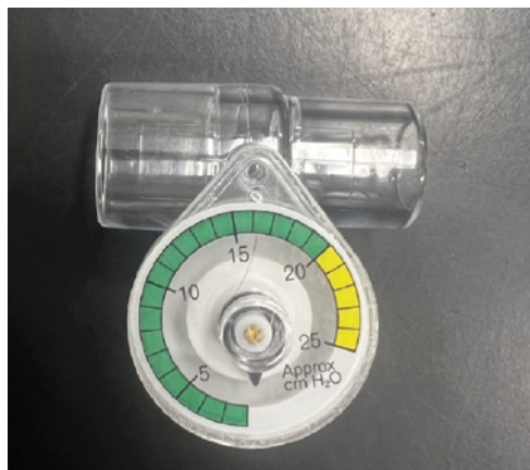
Figure 4.1 A manometer which can be attached to the breathing system to check pressures used while ventilating.
