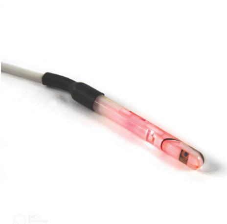
Figure 7.4 Reflectance pulse oximeter probe. Source: Courtesy of Thames Medical®.
