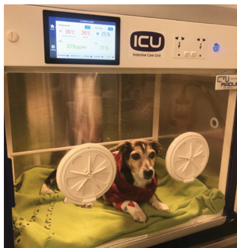
Figure 14.8 An IncuVet® incubator for patient recovery showing warm air temperature and an adjustable FiO 2 for recovery.
