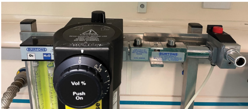
Figure 13.16 A back bar and its components.
