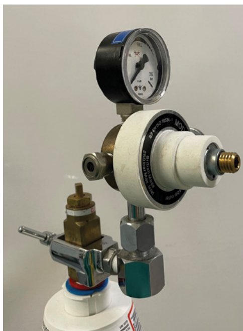
Figure 13.7 Bourdon pressure gauge and pressure reducing valve on top of a cylinder.
