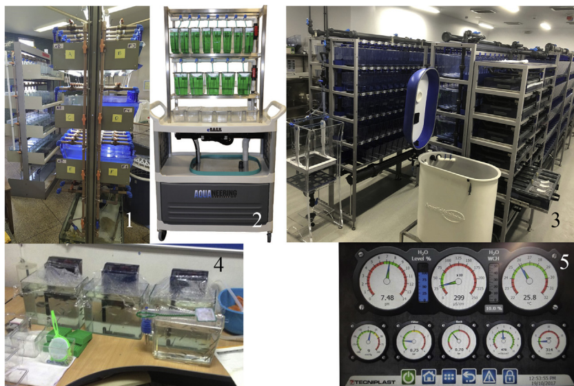
FIGURE 2.2 (1) Two “self-build” recirculating aquaculture systems (RAS) at the Federal University of Jatai, Brazil. Photo Prof. Monica Rodrigues Ferreira Machado. (2) A commercially produced “Educational” standalone RAS. Photo Aquaneering Inc. (3) A large-scale, highly automated rack system with mass spawning devices attached. Photo Bruce Newell, Deakin University. (4) A small zebrafish set-up utilizing “hobbyist” equipment used for approximately 12 months before expansion into a commercially produced RAS system. Photo Dr. Suzita Mohd Noor, Universiti Malaya. (5) Automation control panel monitoring a centralized RAS. Photo Tecniplast SpA.
