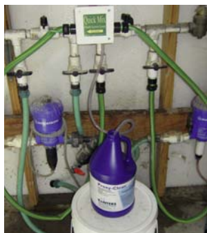
Fig.81.21: Line cleaning using ProxyClean (Hydrogen Peroxide).
