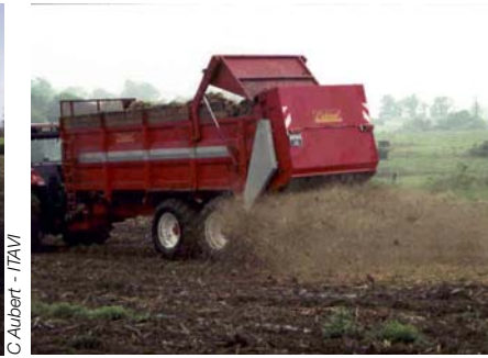
Fig.8.13: Poultry manure spreader with spreading table.
