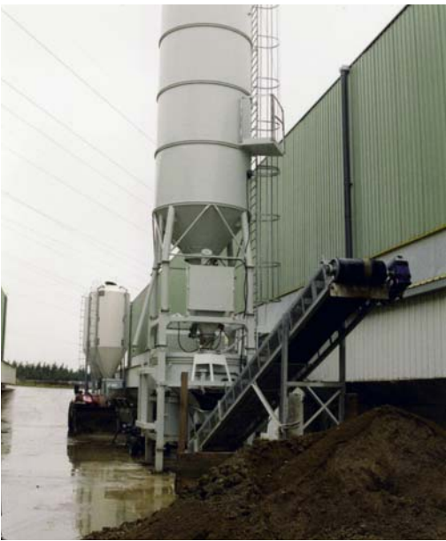
Fig.8.11: Plant for the liming of laying hen droppings.
