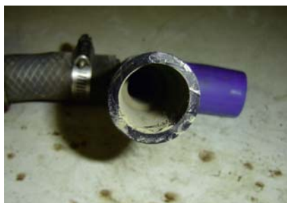
Fig.81.12 &amp; 81.13: The biofilm layer must be peeled off from the drinking system.
