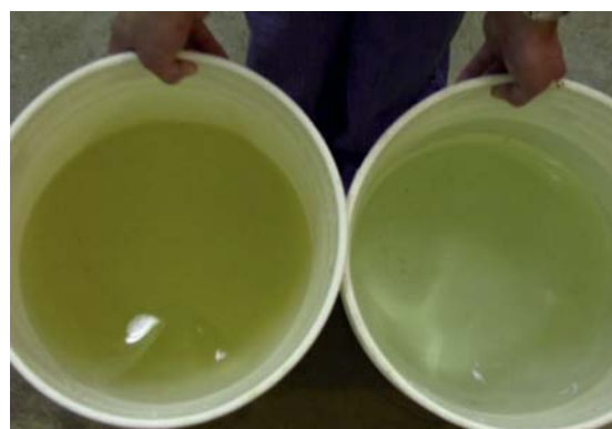
Fig.81.19: Water before and after cleaning water lines.
