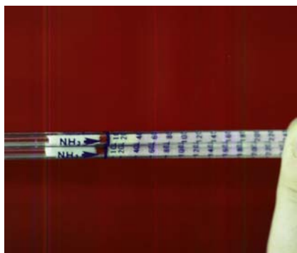
Fig.74.15, 74.16 & 74.17: Assessing ammonia levels in the field.
