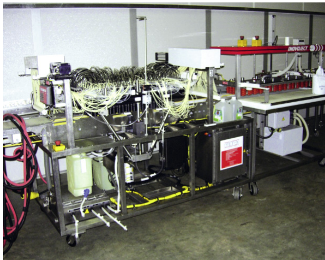
Fig.2.4: In ovo inoculation machine used at transfer from incubator to hatchery.
