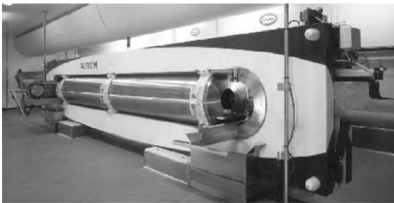
Fig. 16.1 High pressure processing vessel (courtesy of ACB Pressure Systems, France).
