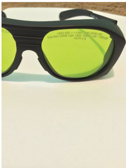
Figure 15.1 Wavelength-specific safety goggles. Note the stamp in the upper corner indicating wavelengths the goggles have been tested and approved for.
