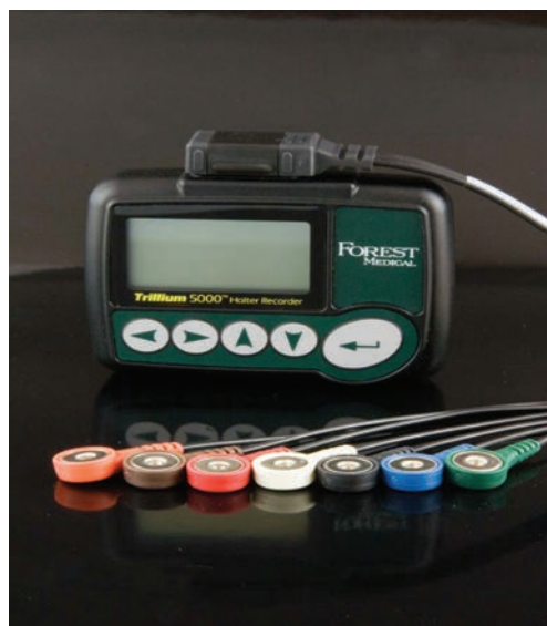
Figure 4.32 A digital Holter monitor with seven cable leads capable of three channel recording. Model is the Trillium 5000. Source: courtesy of Forest Medical, Syracuse, NY.
