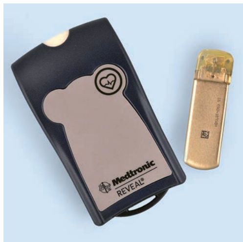
Figure 4.31 An implantable loop recorder (ILR) and the remote control device. The device is approximately 6 \times 2 \times 1 cm and has two exposed metal electrodes on the reverse side. The device is implanted with the electrodes toward the heart under the skin on the thorax. The remote control device allows the client to activate the “save” feature of the ILR should they notice a symptom by pressing the heart diagram on the upper right of the remote.
