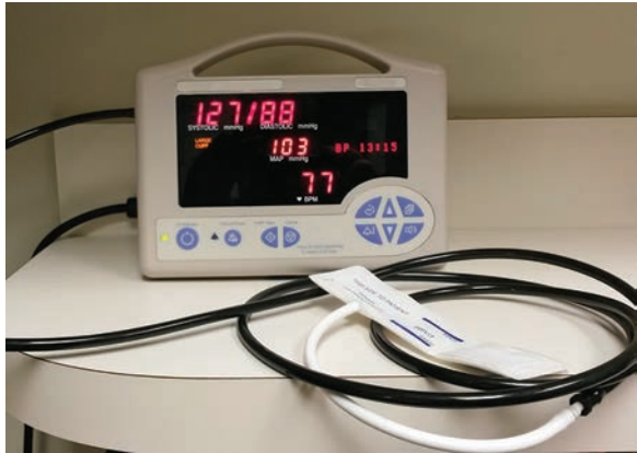
Figure 7.7 An oscillometric blood pressure device showing the systolic/diastolic ABP, the mean ABP, and the pulse rate. The patient cable and cuff can be seen in the foreground. (Cardell 9401 Veterinary Blood Pressure Monitor, CAS Medical Systems, 44 East Industrial Road, Branford, CT 06405, USA. http://www.casmed.com/ .)
