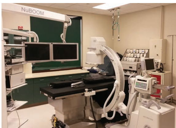
Figure 8.1 Typical fluoroscopy suite. Moving images are displayed on the television monitor and are saved digitally, for playback at regular or slow motion speed. The table is movable in four directions, to allow for constancy of patient position. The unit is operated via a foot pedal.
