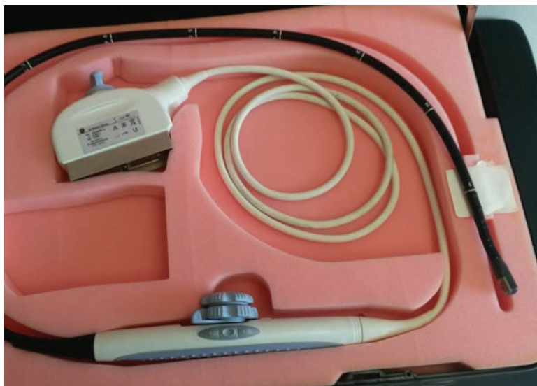
Figure 6.33 A typical transesophageal echocardiographic probe: the transesophageal probe is placed near the heart via the mouth down the esophagus. General anesthesia is required for the procedure. The depicted probe is ~1 m in length and 1 cm in diameter. The control handle allows the operator to bend the tip of the probe in up-down and right-left planes, and rotate the ultrasound crystal head within the tip.
