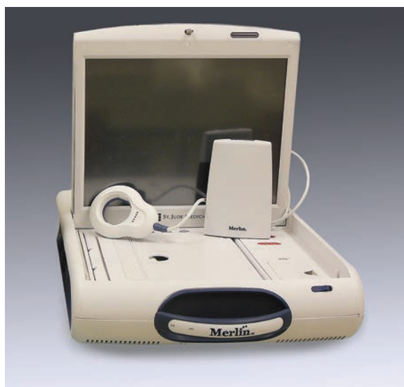
Figure 16.12 An example of a pacemaker programmer. The oval shaped portion (left side) with the circular hole is the “wand” which is held over the pacemaker to allow programming of rate, output, and other parameters. The rectangular tower to the right is the radio frequency antenna that may be used on some pulse generator models.
