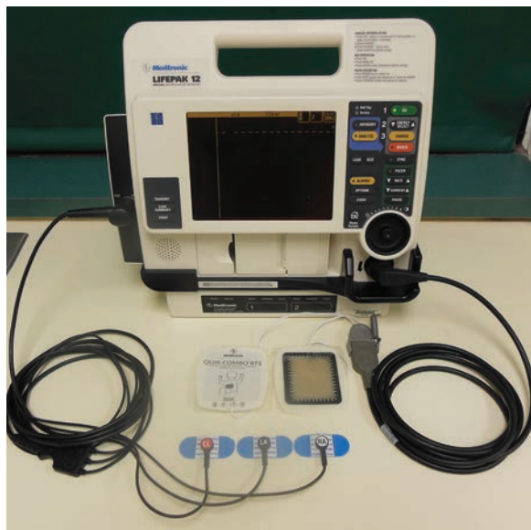
Figure 16.14 A transthoracic pacing system. This device will also function as a defibrillator. The small blue patches shown will provide an electrocardiogram for the system; the larger electrodes just above them are placed on either side of the thorax over the heart. Each side of the pacing patch is shown. The transthoracic pacing system allows control of rate and amplitude only and is for short-term temporary use.
