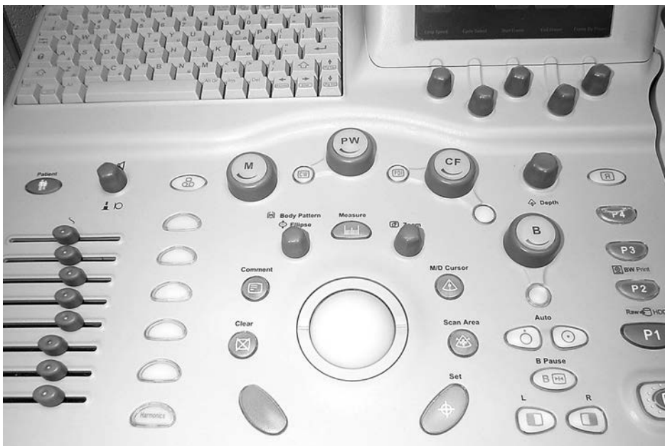
Figure 6.5 Typical echocardiograph console. The slide buttons on the left are the time gain compensation controls. The upper slides control the image gain in the near field. The lower slides control the image gain in the far field. Large knobs labeled M, PW, CF and B, control the M-mode, pulsed-wave Doppler, color-flow Doppler, and standard two-dimensional image, called B-mode, respectively. A small button labeled CW activates the continuous wave Doppler. The track ball in the lower center allows the operator to move a cursor on the screen to make selections that are then activated by the “set” button at the lower right of the track ball. Other controls seen are individual to this console, but similar functions are available on almost every echocardiograph.
