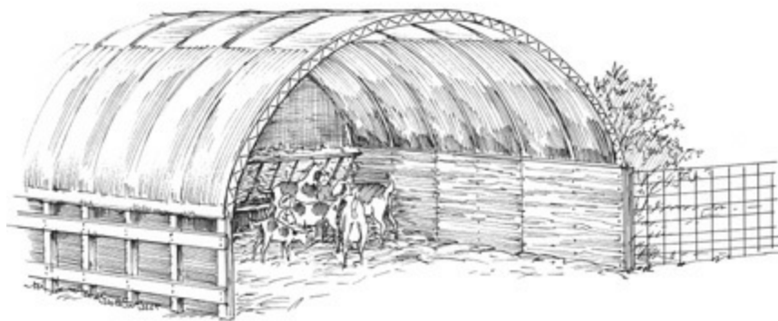
A hoop building supported by a pony wall keeps the canvas safe and shelters the goats with a solid windbreak.
