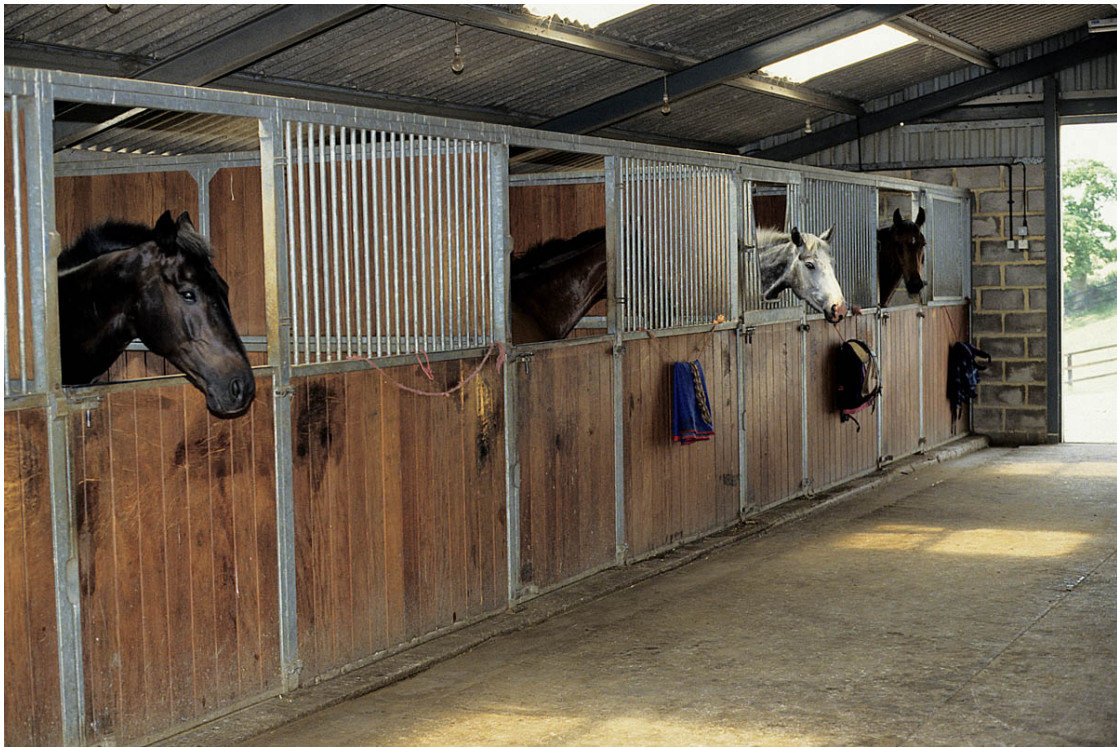
ABOVE: The top of the stall wall or stall door should be made of pipe or metal bars so the horse can see out.
