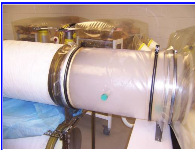
Figure 9.11 The transfer sleeve is fully inflated and feels firm.
