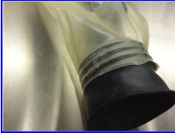
Figure 6.62 The glove and cuff are inserted into the isolator glove port, with the hand of the glove directed toward the isolator and the thumb up.
