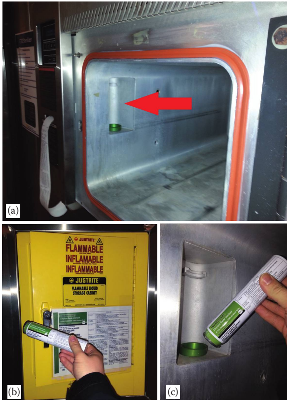
Figure 5.12 Replacing the ETO canister. (a) Ensure that the used canister is removed. (b) Canisters should be stored in a flameproof cabinet. (c) Replace the canister.
