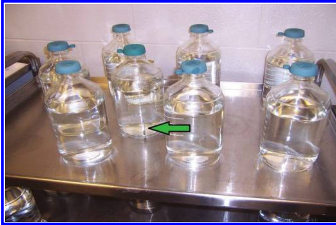
Figure 8.29 Placement of bottles on cart for autoclaving. Steraaffirm® indicator is in the center bottle (arrow).
