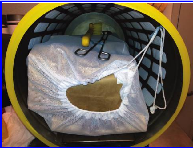
Figure 8.13 Place four bags of bedding on top of feed bags inside mesh bag.
