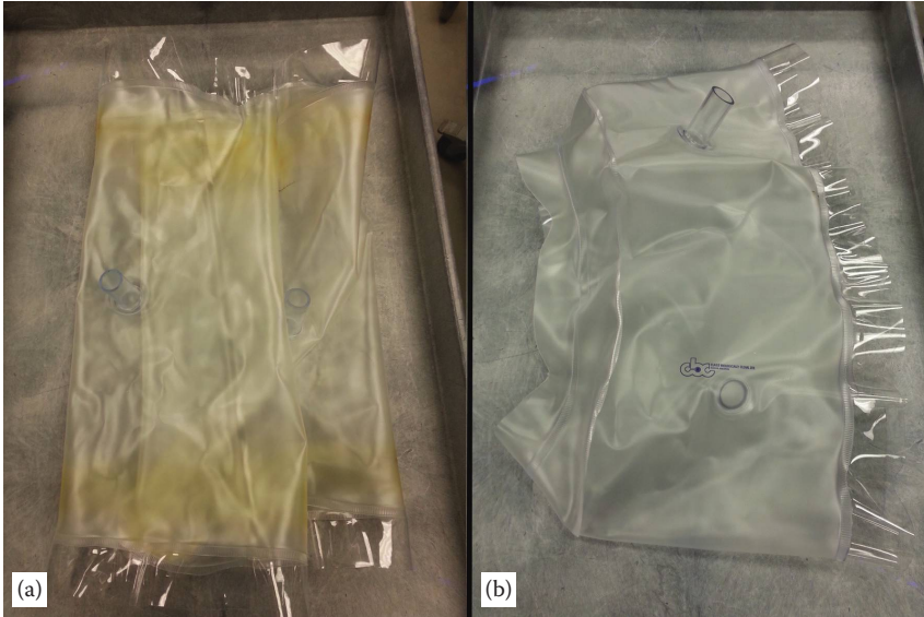
Figure 3.4 Transfer sleeves are used to transfer materials between isolators or from supply cylinders to isolators. We use two types of transfer sleeves: (a) 18"-to-18" sleeves are used to transfer materials between isolators with 18" ports. These sleeves are plastic tubes, 18" in diameter from end to end, and come in various lengths. (b) 18"-to-12" step-down sleeves are 18" at one end and narrow to 12" at the other end. They are used to transfer between isolators with unequal port sizes.
