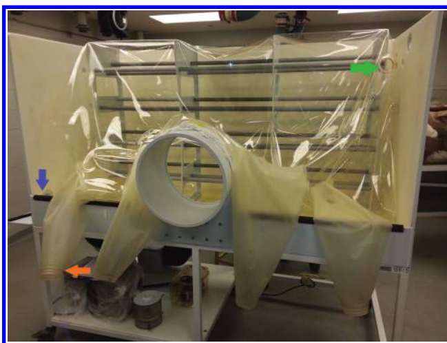
Figure 6.58 Large isolator ready for assembly. At this point, all isolator openings, including the port, the glove openings (orange arrow), the intake filter opening (blue arrow), and the exhaust filter opening (green arrow) are still open.
