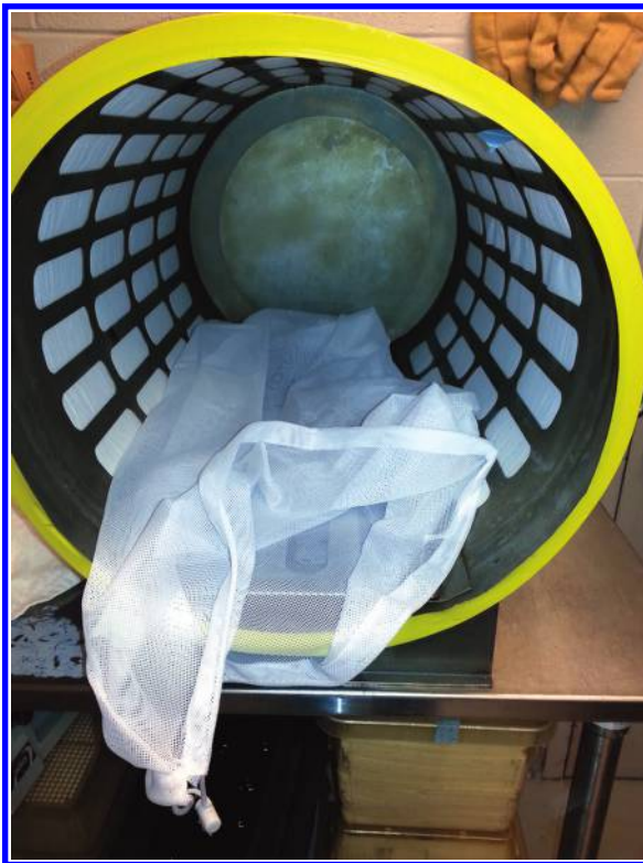
Figure 8.9 Place mesh bag in cylinder.
