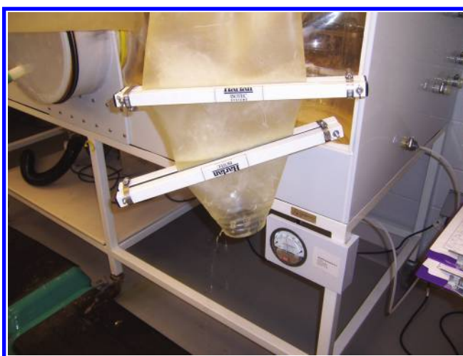
Figure 10.11 Appearance of the clamped sleeve with glove removed. Surface sterilize the surrounding area prior to replacing the glove.
