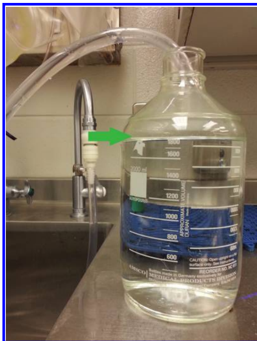
Figure 8.28 Fill 2-L water bottles only to 1800 mL.
