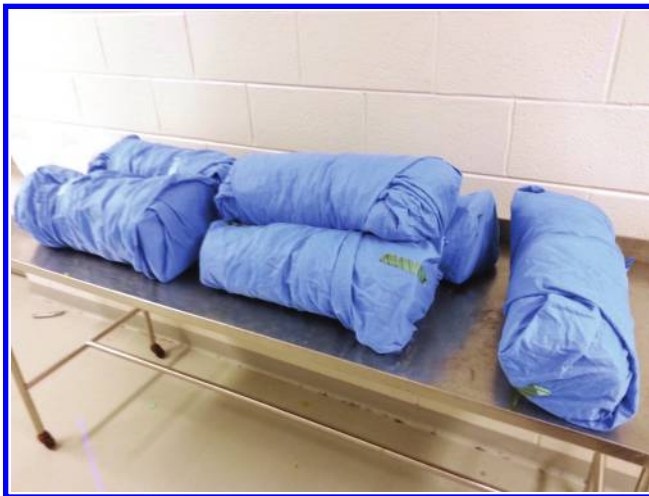
Figure 6.14 Wrapped and autoclaved filters ready for installation.
