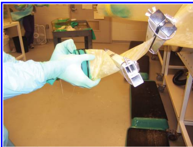
Figure 10.10 Remove the old glove.
