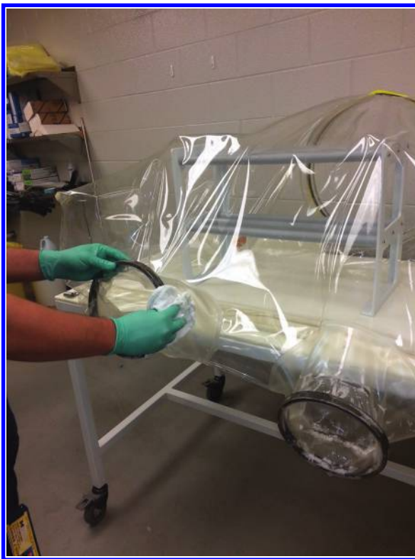
Figure 6.22 After the glove rings are installed, wash the surrounding canopy in preparation for glove installation.
