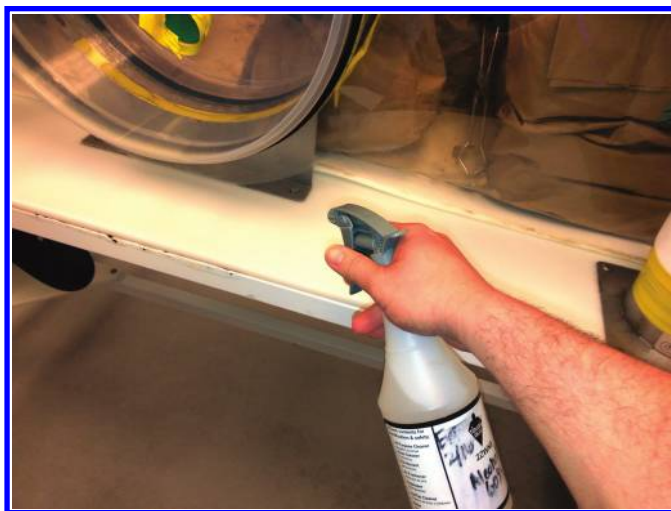
Figure 10.2 Spray isopropyl alcohol to remove chlorine dioxide residue.
