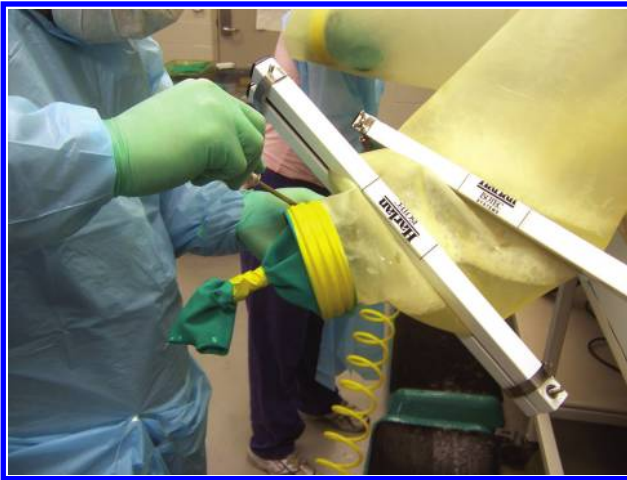
Figure 10.9 Two clamps may be necessary to prevent leakage.
