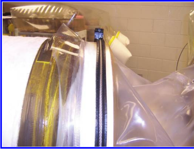
Figure 9.8 Ensure that the sleeve reaches far enough over the cylinder and that it is straight.
