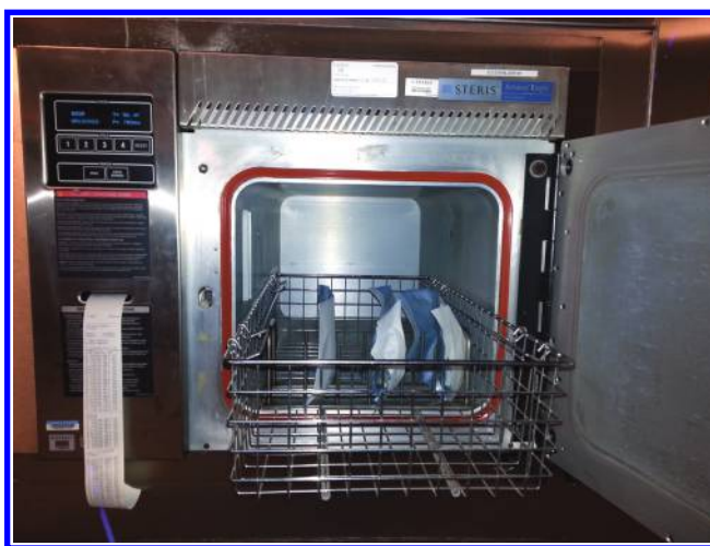
Figure 5.11 Placement of items in the sterilizer.
