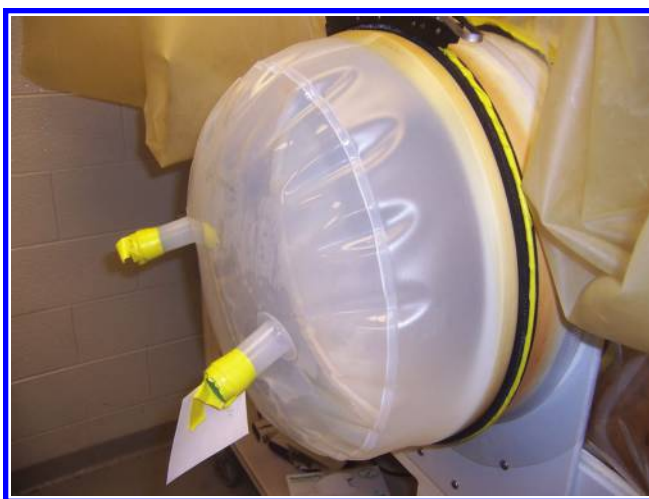
Figure 7.8 Following fogging, the outside cap should remain convex.
