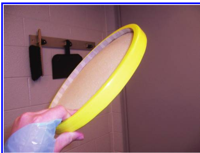
Figure 13.4 Filter disk from shipping container. (For demonstration only: Do not remove the disk or get it wet.)
