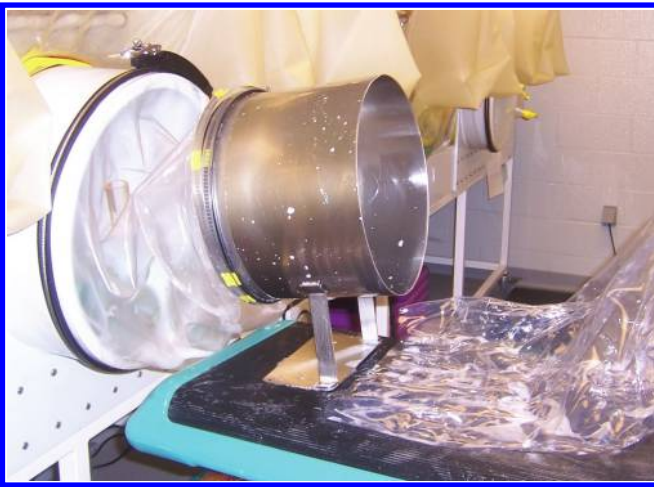
Figure 13.7 Attach the 12" port to the small end of the transfer sleeve.
