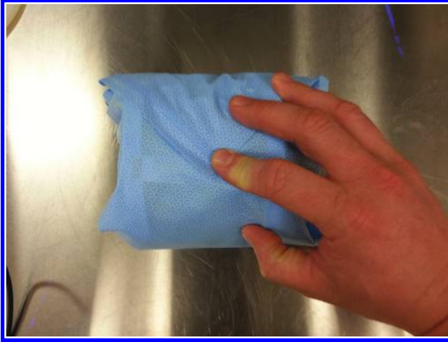
Figure 6.53 Wrapping filters for ETO sterilization; Step 4: Turn the filter around and fold the last, top corner to the center.
