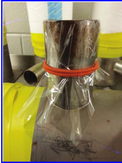
Figure 6.9 Secure with an elastic band.
