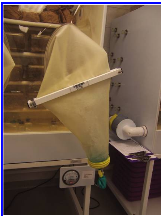
Figure 10.6 The clamp has been placed on the sleeve and the glove taped off with nylon tape.
