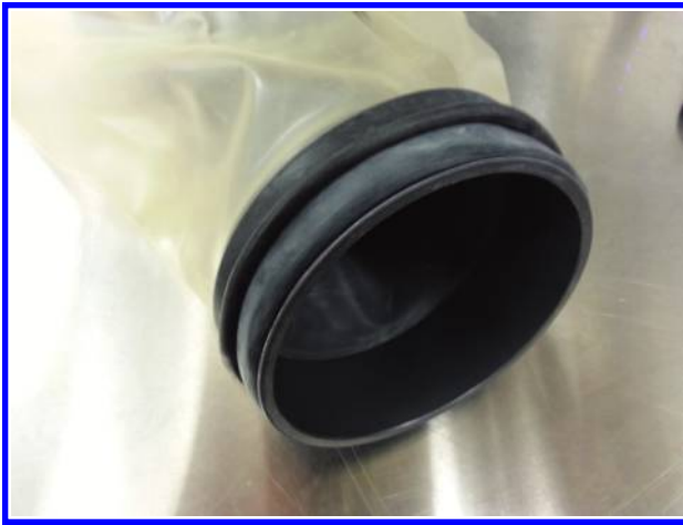
Figure 6.66 Fold the remaining glove material over the second O-ring. Place the third O-ring in the last groove in the middle.
