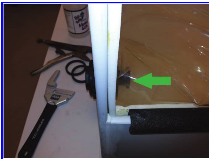
Figure 6.70 Interior, threaded plug (green arrow).
