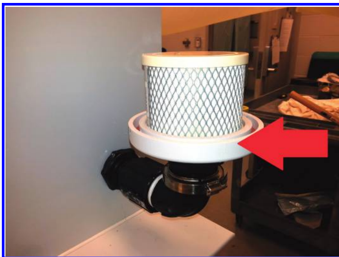
Figure 6.80 Intake filter and bottom component of filter housing installed in the 90° fitting assembly.
