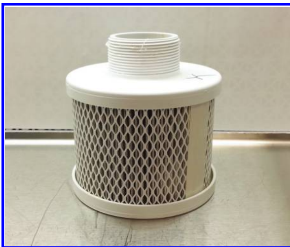
Figure 6.47 Intake filter frame for large isolators.
