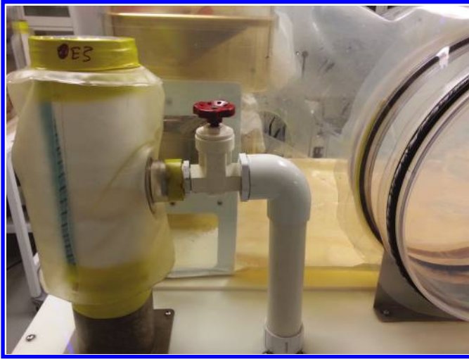
Figure 6.42 Filter bag placed around intake filter.
