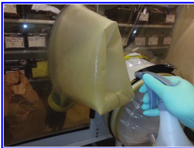
Figure 10.4 Use isopropyl alcohol to clean the inside of the glove sleeve.
