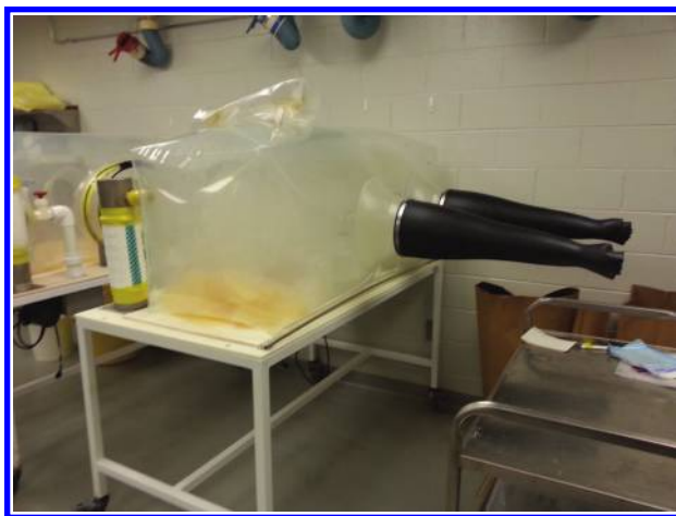
Figure 6.38 Fully inflated isolator filled with vaporized sterilant. Note horizontal position of gloves.
