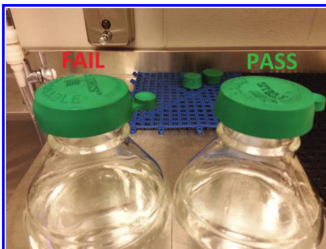
Figure 8.31 Sealing of sterilized bottles is indicated by a dip in the green cap (right). Absence of a dip (left) indicates seal failure.
