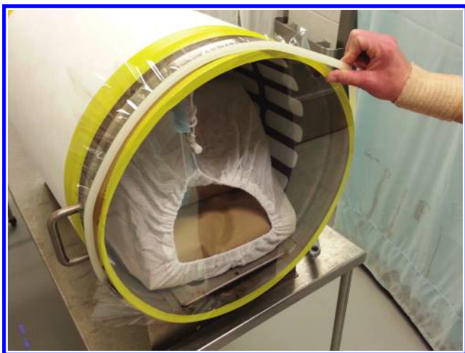
Figure 8.17 Remove the silicone band. Film is held on with the rubber band.
