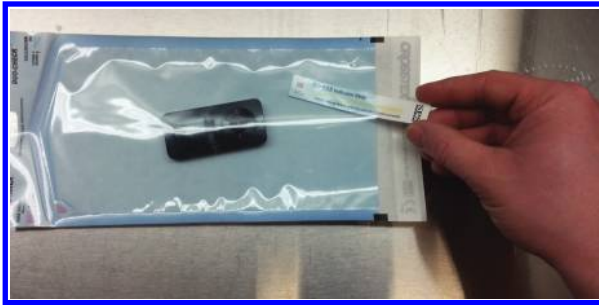
Figure 5.9 Entering item to be sterilized and indicator strip into the peel pouch.
