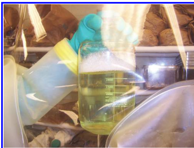
Figure 10.7 From inside the isolator, pour the sterilant into the sleeve.
