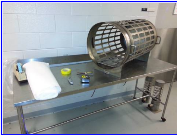
Figure 8.5 Cylinder frame, HEPA media, and materials for assembly.
