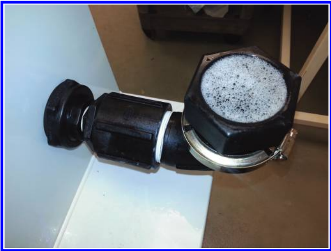
Figure 6.77 Fill the 90° fitting assembly with sterilant.
