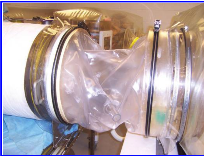
Figure 9.9 The transfer sleeve is clamped to the port on one end and the cylinder on the other end.
