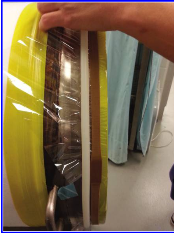
Figure 8.16 The film overlaps itself around the edge of the cylinder. This is commonly where pinholes form.
