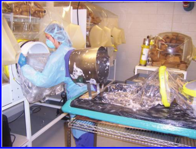
Figure 13.6 Place the transfer sleeve on the isolator port.
