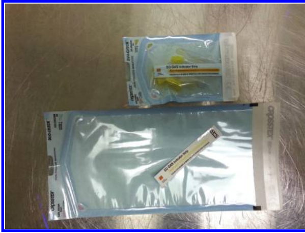
Figure 5.8 Peel pouches with indicator strips. The top pouch contains sterilized tubes and a processed indicator strip. The bottom pouch contains an unprocessed strip.
