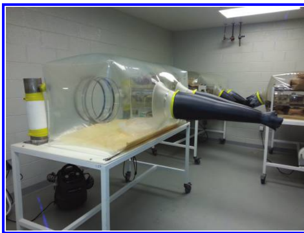
Figure 6.39 Leak test. At the end of an hour, the gloves should remain at or close to their original horizontal position.
