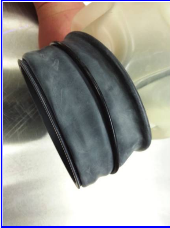
Figure 6.65 Place another (second) O-ring on the furthest groove of the cuff from the glove opening.
