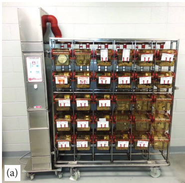
Figure 2.3 (a) Tecniplast ISOcage P rack designed to deliver HEPA-filtered air to cages via a sealed system. (b) Individual ISOcage. The cage is airtight and seals when removed from the rack, essentially acting as a self-contained germ-free isolator.
