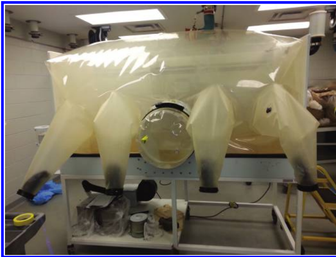
Figure 6.89 Partially inflated isolator.
