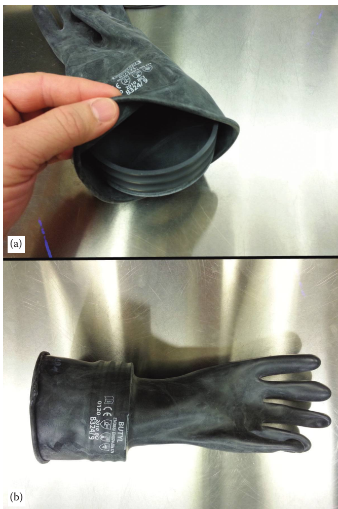
Figure 6.61 (a) Fit the cuff into the glove. (b) The cuff should be inserted into the glove for approximately twice its width.
