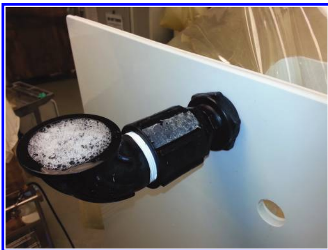
Figure 6.74 The 90° fitting assembly installed and filled with sterilant.
