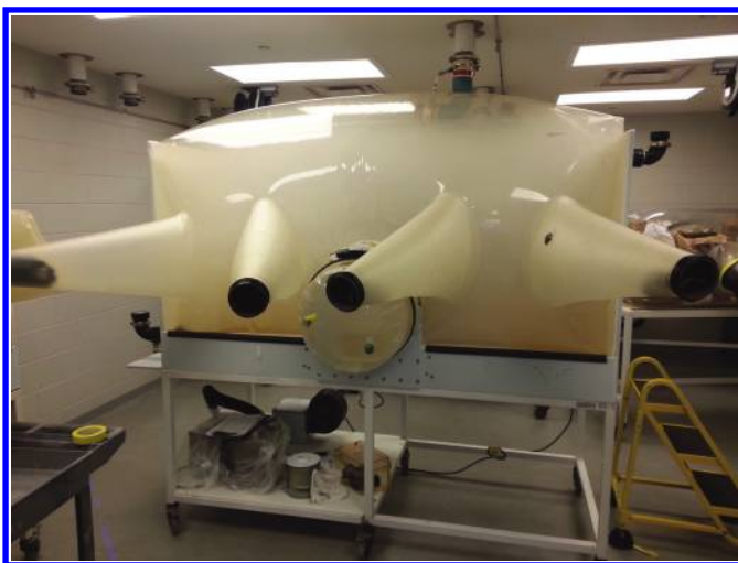
Figure 6.87 Fully inflated isolator after leak test.
