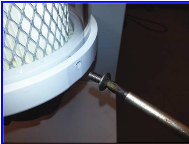
Figure 6.82 Secure the filter housing with screws.
