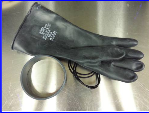
Figure 6.59 Components for installing gloves: gloves, three O-rings, and cuff.
