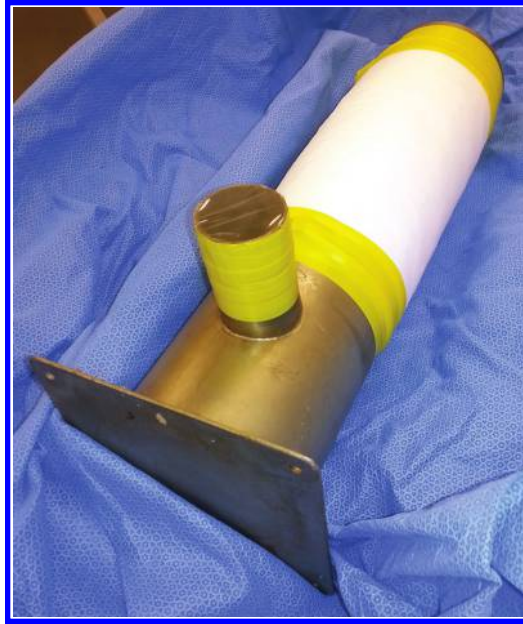
Figure 6.13 Wrap the filter for autoclaving.
