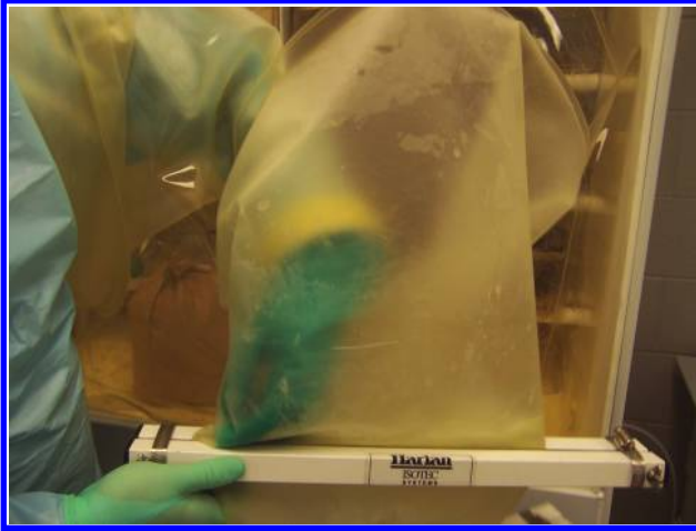
Figure 10.8 Ensure that the sterilant reaches all surfaces.
