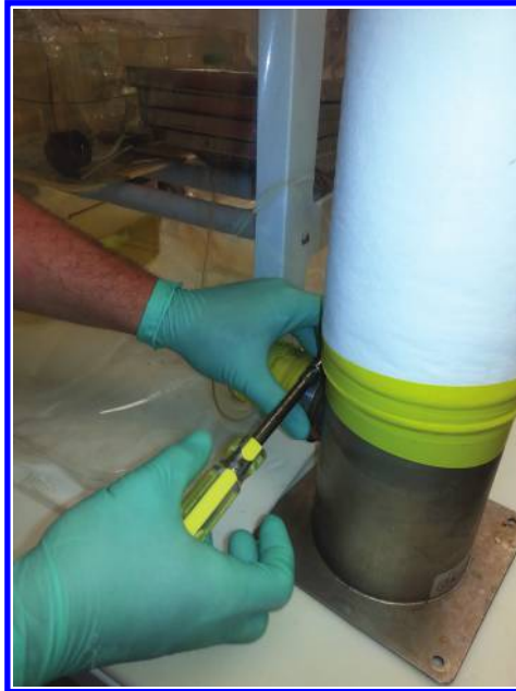
Figure 6.34 Tighten the clamp.
