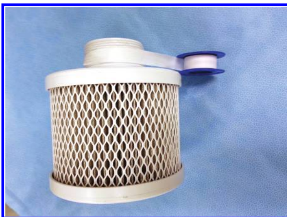
Figure 6.48 Wrap the filter threads with plumber's tape.
