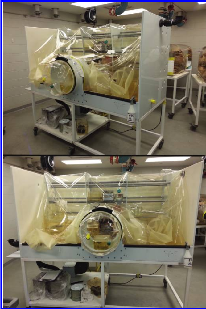
Figure 6.75 Two views of partly assembled isolator prior to stocking supplies.
