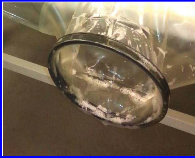
Figure 6.23 Glove hole with glove rings inserted.
