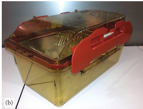
Figure 2.3 (a) Tecniplast ISOcage P rack designed to deliver HEPA-filtered air to cages via a sealed system. (b) Individual ISOcage. The cage is airtight and seals when removed from the rack, essentially acting as a self-contained germ-free isolator.
