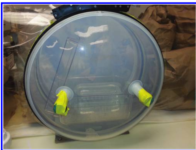
Figure 7.9 Proper placement of items in the port ensures optimal contact with vaporized sterilant.
