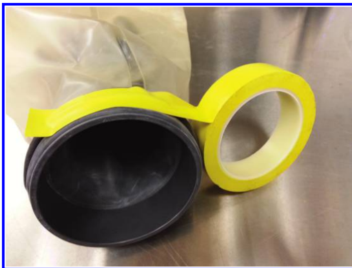
Figure 6.67 Use nylon tape to cover the glove material and edges of the cuff.
