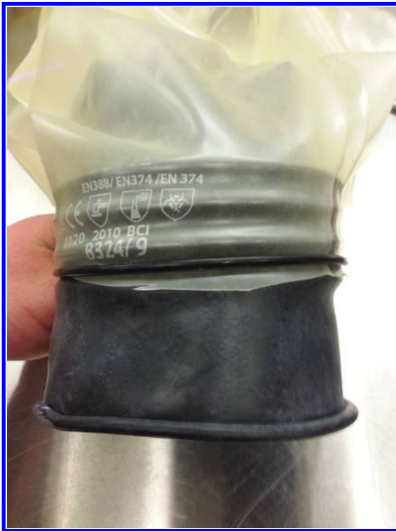
Figure 6.63 Place an O-ring into the last groove (closest to the opening of the glove), securing the end of the glove port to the glove and cuff.
