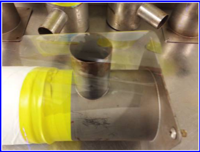
Figure 6.8 Place polyester film over the filter opening.
