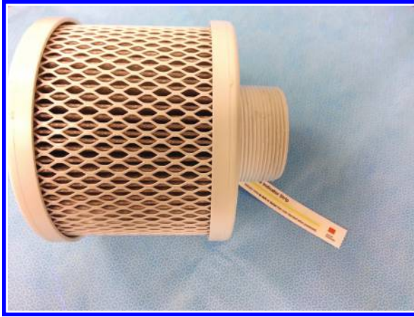
Figure 6.49 Place the filter frame and ETO sterilization strip on a blue wrap.
