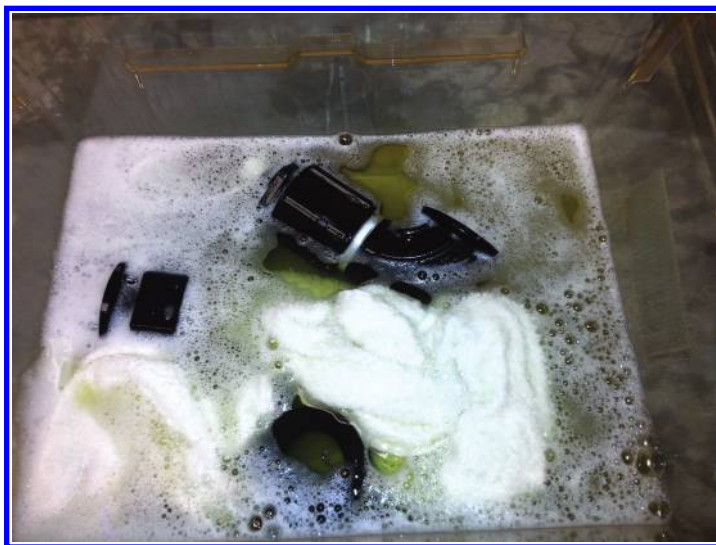
Figure 6.68 Soak the autoclaved pipe fittings in sterilant.
