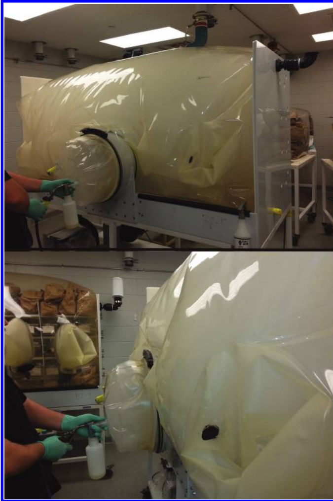
Figure 6.85 Adjust the canopy as the isolator inflates.
