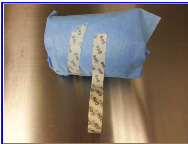
Figure 6.55 Unprocessed (brown) and processed (green) ETO indicator tape.
