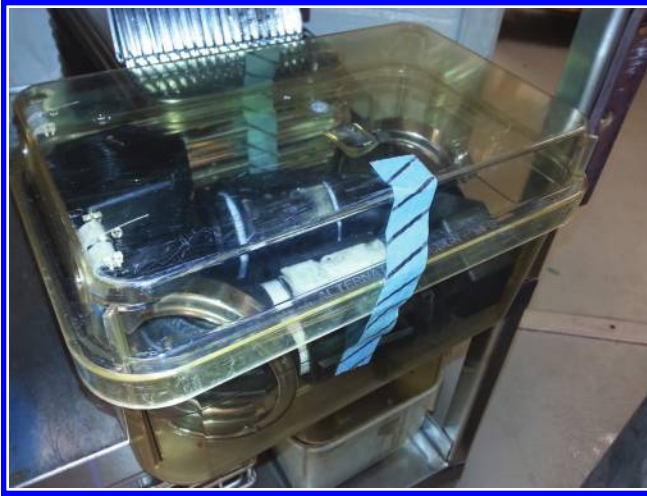
Figure 6.56 Filter piping packed for autoclave.
