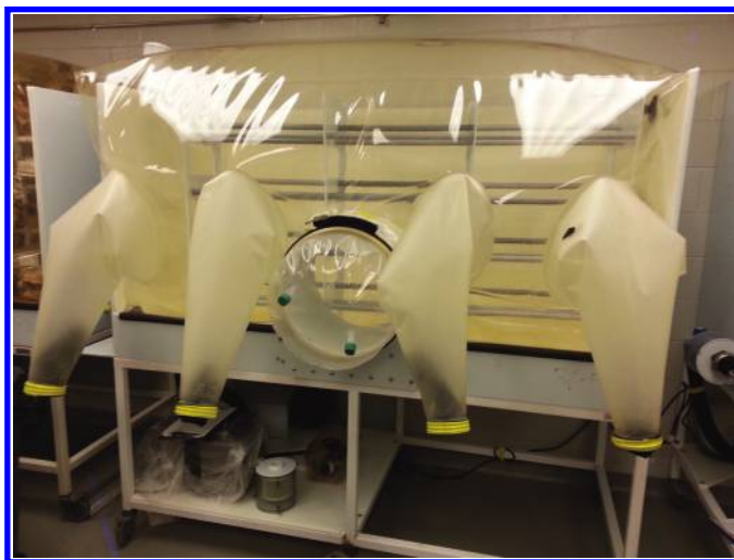
Figure 6.46 Large breeding isolator made by CBClean.
