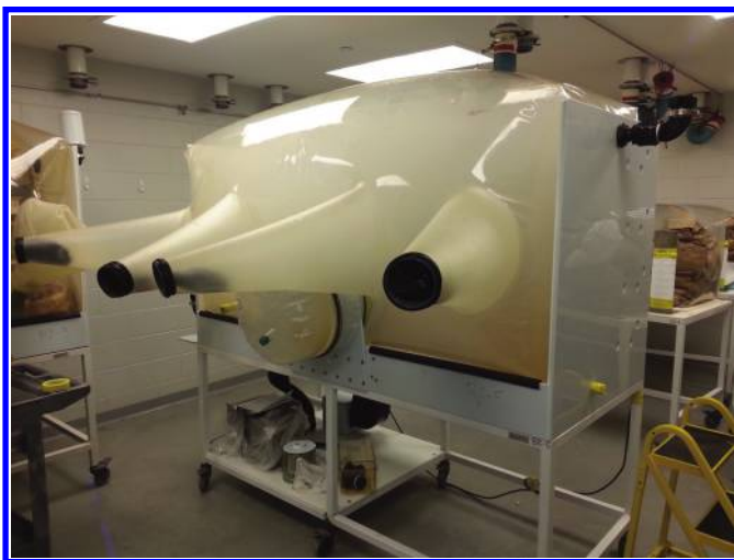
Figure 6.86 Fully inflated isolator.
