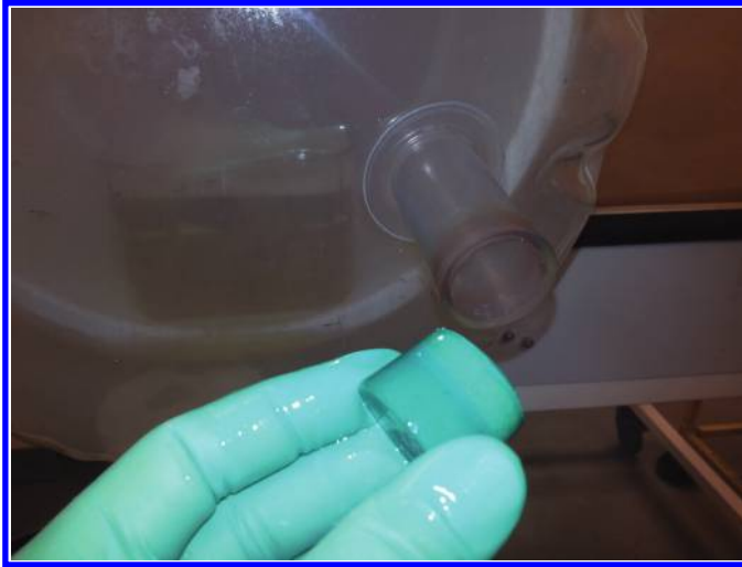
Figure 6.88 Remove one rubber stopper.
