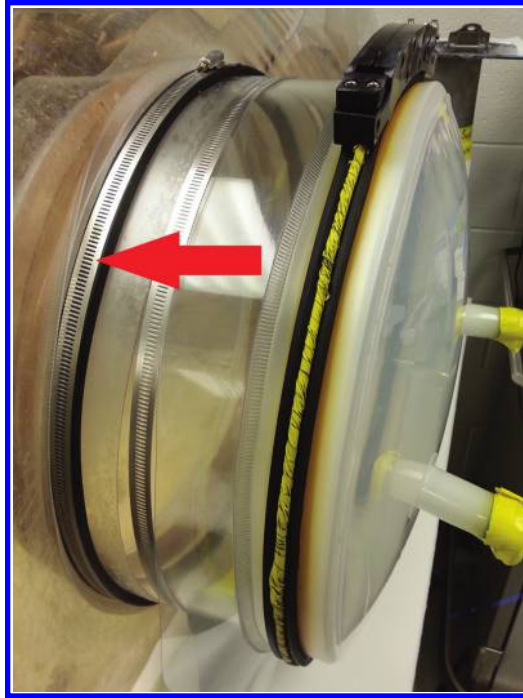
Figure 6.20 Assembled canopy and port. Cover the clamp (red arrow) with nylon tape.
