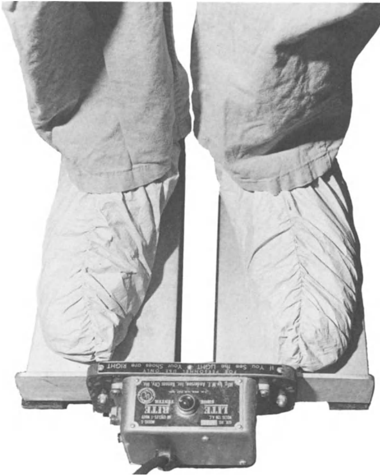
Figure 3. The conductivity of the shoe covers is tested by standing on a conductivity tester.
