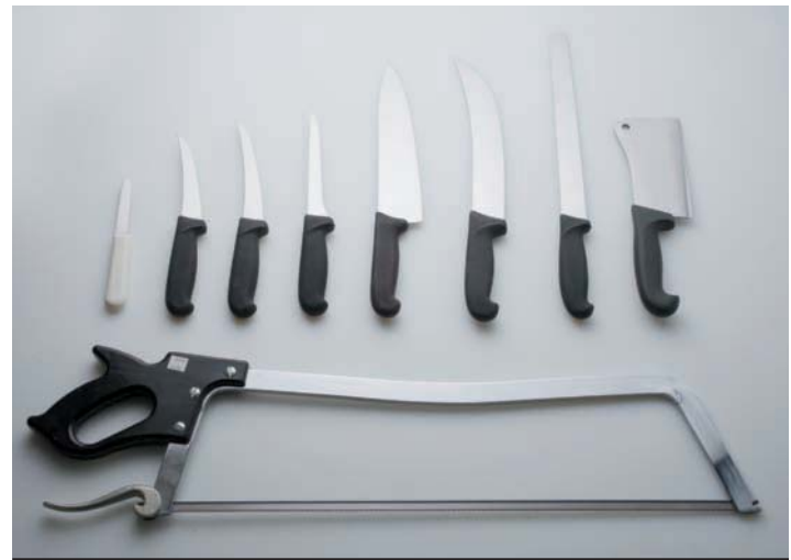
FIGURE 1.6 Top row, from left to right: Clam knife; five-inch curved, flexible boning knife; six-inch curved, flexible boning knife; six-inch stiff boning knife; ten-inch chef's knife; ten-inch scimitar; twelve-inch slicer; cleaver; Bottom row: 25-inch handsaw.
