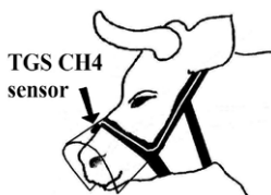
Figure 1. Sketch of the position of the CH 4 -specific TGS sensor under a nose-screen.
