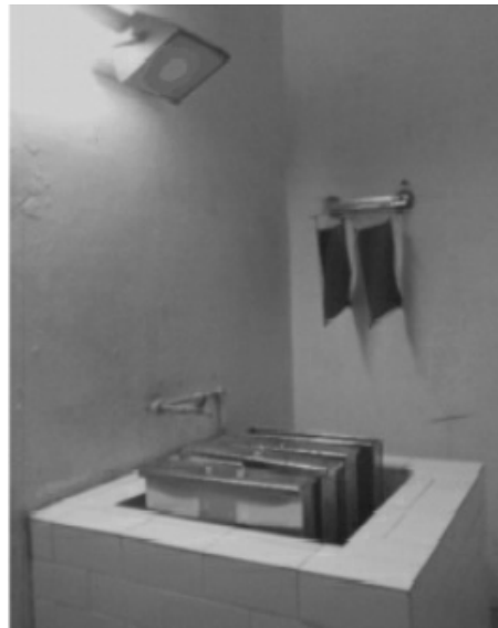
Fig. 12.2: Wet side of dark room showing safe light, processing tanks and film drying rack with film hangers
