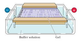
**FIGURE 13.2** The experimental setup for gel electrophoresis. The samples are placed on the left side of the gel. When the current is applied, the negatively charged oligonucleotides migrate toward the positive electrode.
