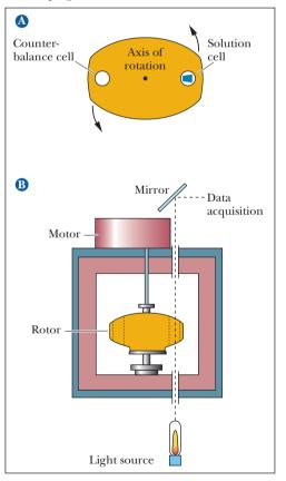
■ **FIGURE 9.25** The analytical ultracentrifuge. (a) Top view of an ultracentrifuge rotor. The solution cell has optical windows; the cell passes through a light path once each revolution. (b) Side view of an ultracentrifuge rotor. The optical measurement taken as the solution cell passes through the light path makes it possible to monitor the motion of sedimenting particles.
