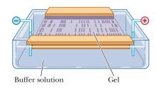
**FIGURE 5.10** The experimental setup for gel electrophoresis. The samples are placed on the left side of the gel. When the current is applied, the negatively charged molecules migrate toward the positive electrode.
