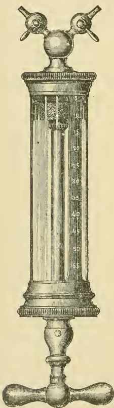
FIG. 198.—Double-acting syringe.
