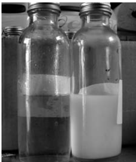
Fig. 3.5 The effect of adding coagulant and polymer during the treatment of wastewater.
