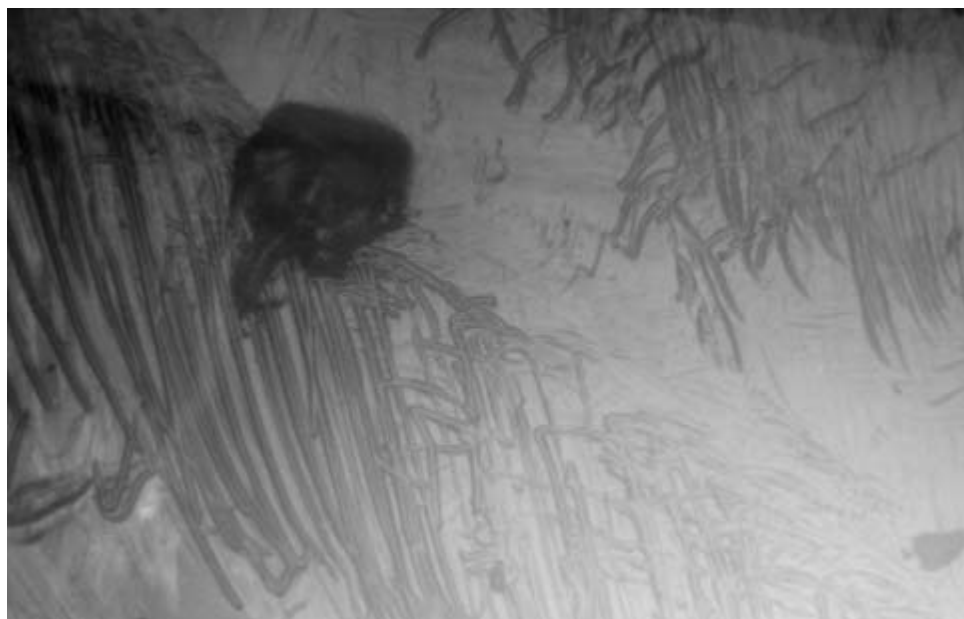
Fig. 10.9 Micrograph showing heat blisters on a UF membrane. Reproduced by permission of JohnsonDiversey Ltd, Northampton, UK.
