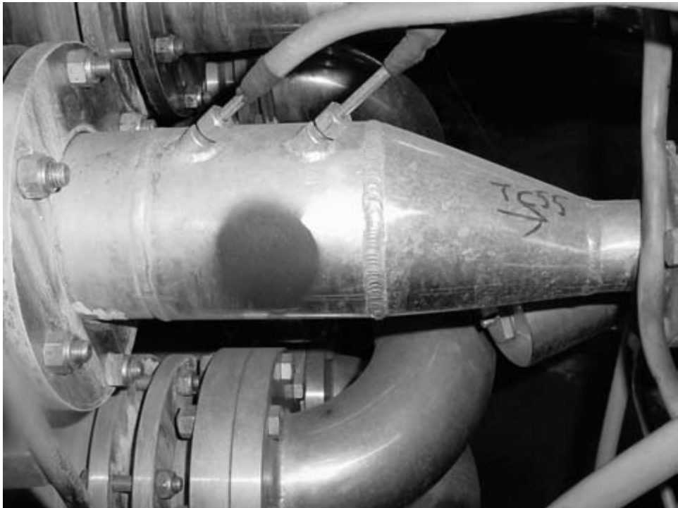
Fig. 8.2 Double Pt100 thermocouple positioned at a tube outlet. Reproduced by permission of Unilever R&D, Bedford, UK.
