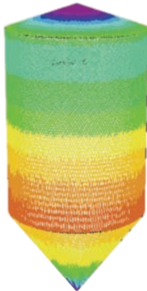
Plate 3 SaniJet 25 – full pattern of cleaning liquid distribution build-up. Reproduced by permission of Alfa Laval Tank Equipment A/S, Ishoej, Denmark.
