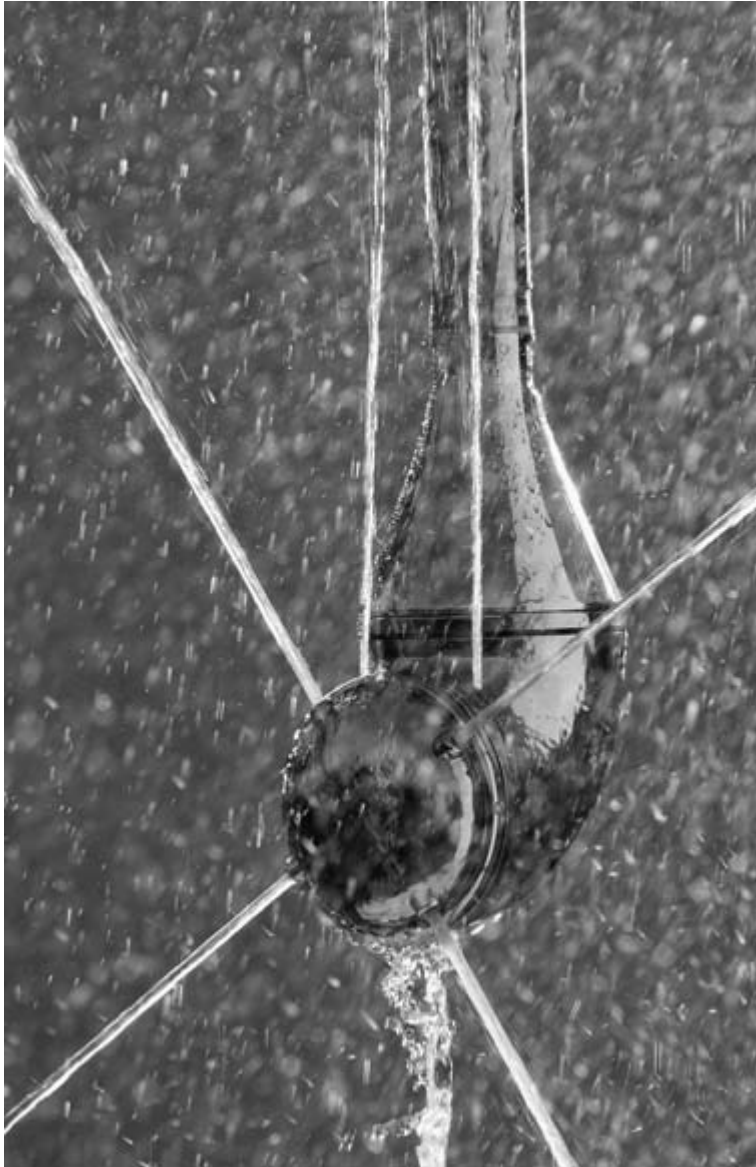
Fig. 6.11 A rotary jet head distributing the cleaning liquid through four nozzles – SaniJet 25. Reproduced by permission of Alfa Laval Tank Equipment A/S, Ishoej, Denmark.
