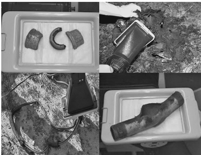
Figure 6.1 (See Color Insert.) An STU-100 scent collection from a detonated bomb and arson evidence. (Photos courtesy of William Kift.)
