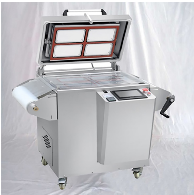
FIG. 10.9 Manually operated gas flushing MAP for a four-tray sealing machine.
