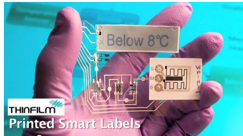
FIG. 10.28 SmartLabel from ThinFilms (Norway); integrated screen shows temperature. https://venturebeat.com/2012/12/19/thin-film-electronics-demonstrates-a-way-to-make-disposable-interactive-smart-labels-that-replace-bar-codes/ .
