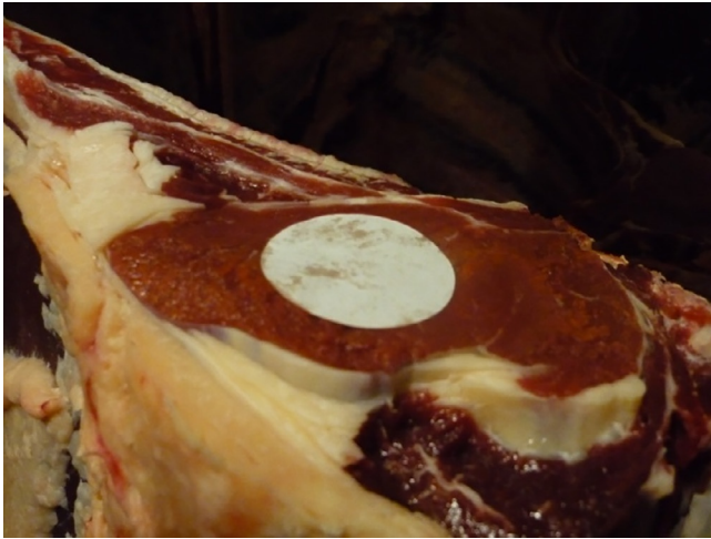
FIG. 14.17 Illustration of the rapid filter method for measuring weep or exudate on a beef loin surface. The filter paper can either be weighed, for amount of fluid absorbed, or scored for % of wetness. Credit: Athula Naththarampatha, Department of Primary Industries, Victoria, Australia.
