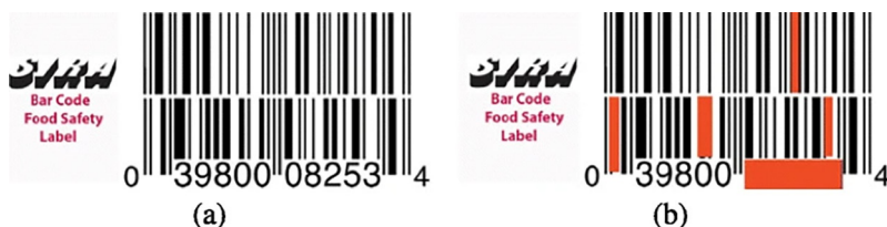
FIG. 10.22 Food Sentinel Systems barcode (Sira). (A) Ready to use; (B) product expired and code is unscannable.
