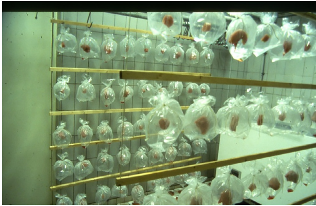
FIG. 14.16 Illustration of the gravimetric method for measuring drip loss, involving suspension of a meat sample in an inflated bag, and storage at 2–4°C for 1–2 days. Credit: Robert Kauffman, University of Wisconsin-Madison.
