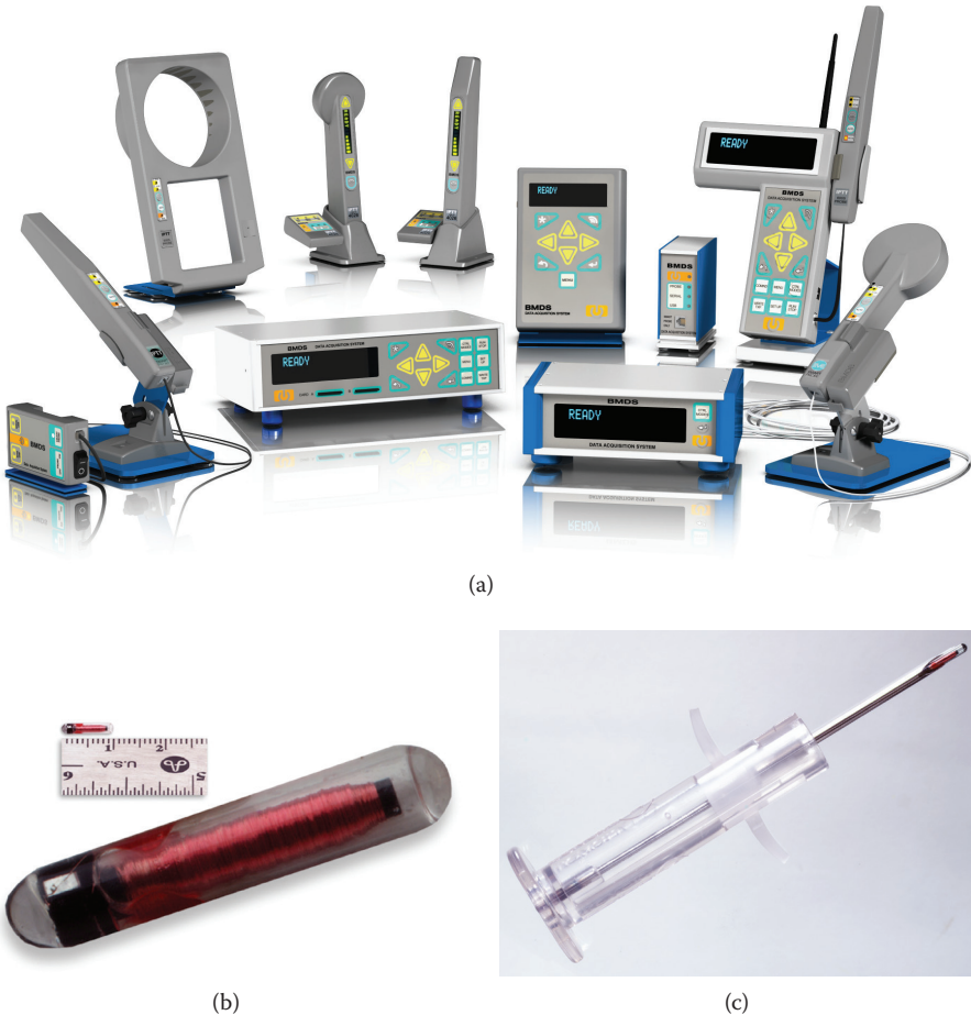
Fig. 29 (a) Electronic transponder readers. (b) Microchip transponder (actual size and high magnification view). (c) Microchip transponder in a trochar ready for implantation. (Image (a) courtesy of Bio Medic Data Systems, Inc.; images (b) and (c) courtesy Trovan, Ltd.)
