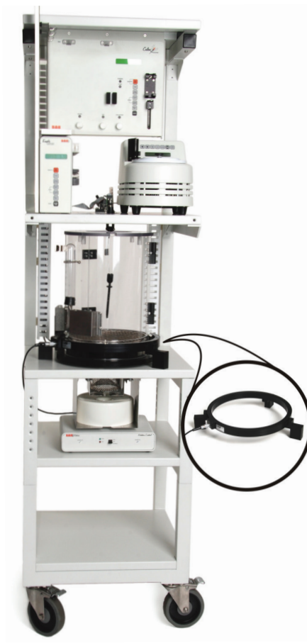
Fig. 60 Automated Blood Sampling with Telemetry unit. 495 mm × 495–953 mm × 1778 mm.
