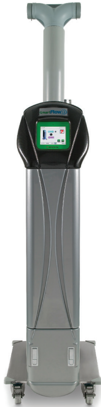
Fig. 12 Tower blower unit. Tower blower units are an alternative to wall, interstitial, and rack-mounted systems. The tower blower occupies valuable floor space that would otherwise house an additional vertical column of rat cages on an IVC rack. Dimensions: 330 × 658 × 1926–2086 mm. (Image courtesy Tecniplast.)
