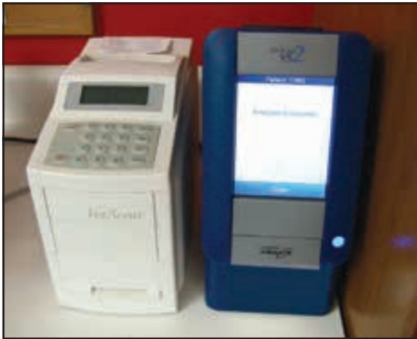
20.2 The advantage of in-house diagnostic testing is speed of results. An additional benefit of this unit is the ability to produce reliable results with at minimum 0.15 ml high quality whole blood. (Courtesy of IDEXX Abaxis, Union City, California.)
