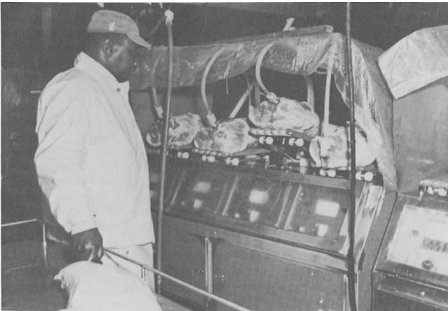
FIG. 3-3. Artery cure pumping operation. Courtesy of the National Provisioner, Chicago, Illinois.
