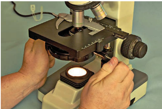
Fig. 6.14. Aligning the phase rings of the phase microscope.
