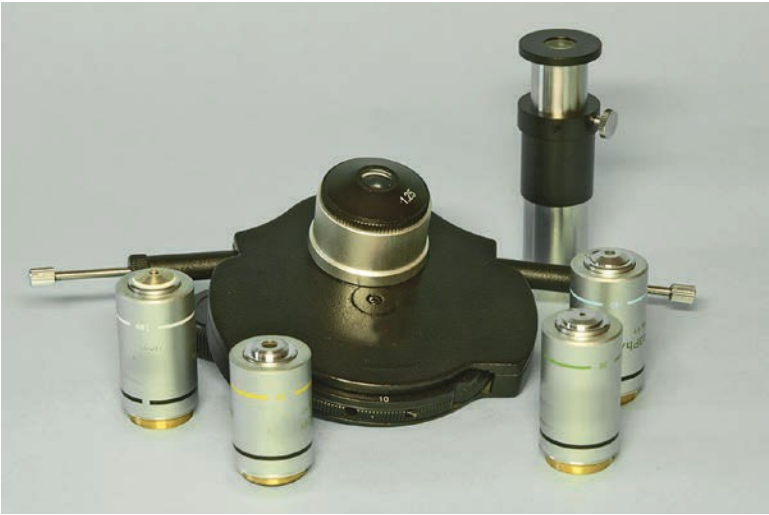
Fig. 6.9. The components of the phase microscope system: phase turret condenser (centre), phase objective lenses (four, bottom) and centring telescope (top right).
