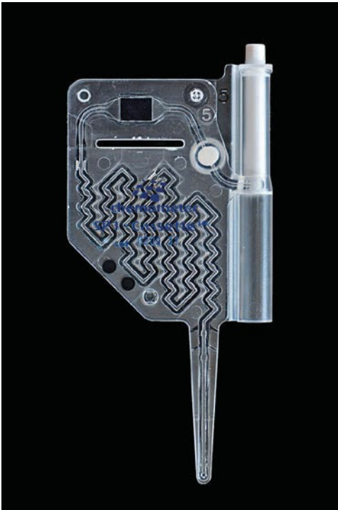
Fig. 6.6. The NucleoCounter® SP-100™ cassette. Note the two black dots on the cassette. During manufacture, the depth of the analysis chamber (upper centre of the cassette) is measured using a laser. The number and location of the black dots on each cassette are evaluated before concentration analysis and represent a final calibration of sample volume in the analysis chamber. Photo by L. Lorton.
