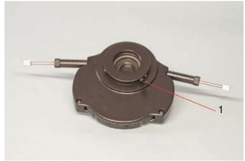
Fig. 6.12. The phase condenser of the phase microscope with the diaphragm control lever (1) shown upside down.
