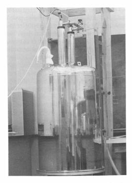
Figure 23–25 A 5-in. bore superconducting magnet
