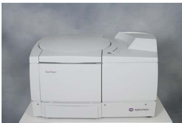
Fig. 4.3 Rapid sequencing of the viral genomes. QuanTyper™-48, from AlphaHelix Molecular Diagnostics AB, is the first real-time thermo cycling instrument utilizing SuperConvection™ to speed up the cycling process. This is achieved by subjecting the samples to high g-force, (via centrifugation), while cycling the temperature. The result is an increased mixing of the sample fluid that improves both the temperature homogenization and the kinetics of the reaction. This makes the QuanTyper-48 very fast but also very flexible with a vast sample volume range, accommodating reactions from 20 to 200 \mu\text{L} in volume using standard PCR-tubes. Typically a 20 \mu\text{L} real-time PCR assay is ready within 15 min while a 200 \mu\text{L} reaction takes up to 50 min to complete. Since such viruses can also be important factors in various diseases, it is important to work on methods, which facilitate their detection
