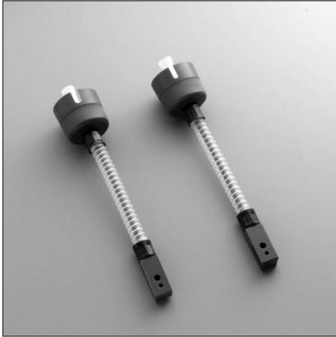
Figure 3-14A Key Fill Adaptors. In addition to color coding, caps on fill spouts are designed to accept knobs specific for each inhalation anesthetic. Courtesy of Matrx, Orchard Park, NY
