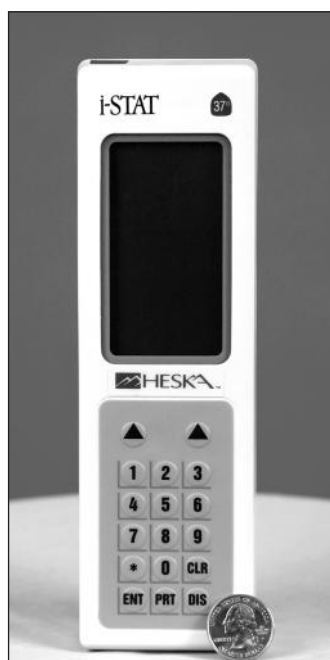
Figure 4-26 Photograph of the iSTAT® hand-held blood gas analyzer. Size is referenced to a quarter.
