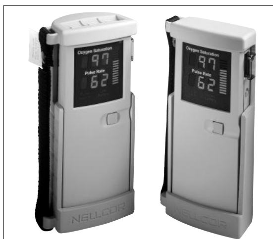
Figure 4-24 Nellcor Model N20 Pulse oximeters. Oxygen saturation is indicated at the top, pulse rate at the bottom. The indicator on the right side of the screen rises and falls with each pulse. On some monitors, the wave form is shown across the screen.
