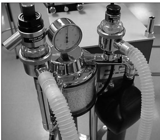
Figure 3-30 Anesthtic machine with APL valve mounted on dome valve positioned between the exhaust (expiratory) valve and CO 2 absorber.
