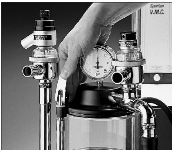
Figure 3-27 Lever-Cam on CO 2 absorber is used to facilitates changing of absorbent or prepack canister replacement. Courtesy of Matrix, Orchard Park, NY
