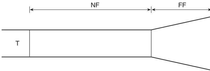
Figure 1.6a This diagram shows the shape of the unfocussed ultrasound beam as it emerges from the transducer with a narrow near field (NF) and a diverging far field (FF).
