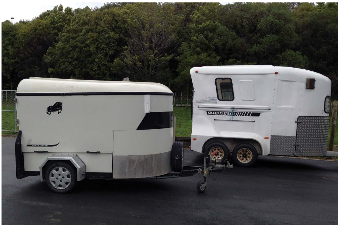
Fig. 8.2 Forward facing two-horse trailers (floats). Note, the float in the foreground has been built using a non-reinforced utility trailer chassis. This latter design is not recommended by the authors. Photo: C.B. Riley.
