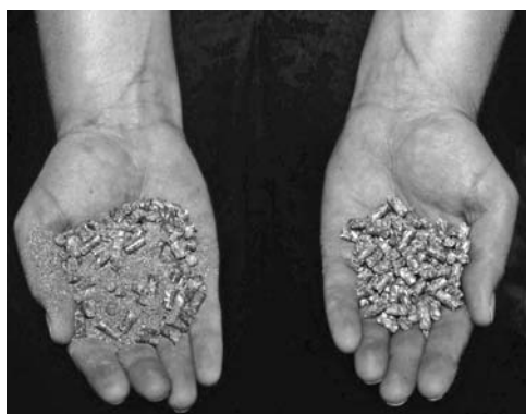
Fig. 7.11. An example of a pelleted diet with excessive fines (left) compared with good-quality pellets (right). (Courtesy of P.R. Cheeke)
