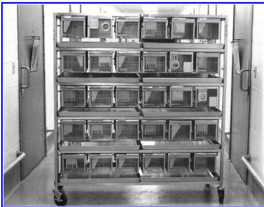
Figure 3.2 Rack of suspended wire mesh cages.
