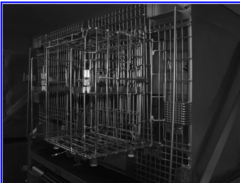
Figure 9.8 Procedure cage mounted to the front of an individual cage in a standard two-by-two rolling rack.
