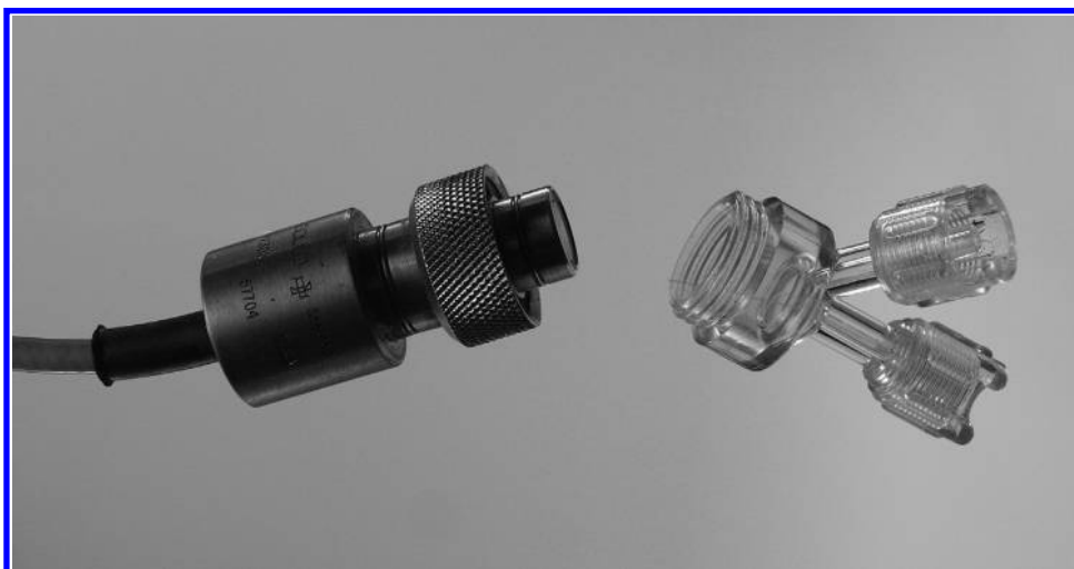
Figure 13.3 Statham pressure transducer: The pictured transducer has a thin metal membrane that is connected to a Wheatstone bridge. The plastic dome covers the membrane and allows connection of a fluid-filled cannula and a flush port to remove all bubbles from the system and keep the cannula clear of blood clots.
