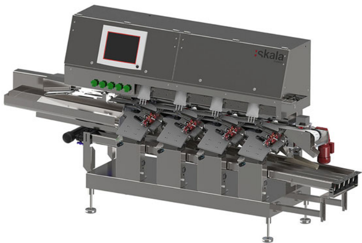
Fig. 19.1 Fully automated vaccination machine used in large-scale salmon smolt farms. https://www.skalamaskon.no/aquakultur/vaksinerings
