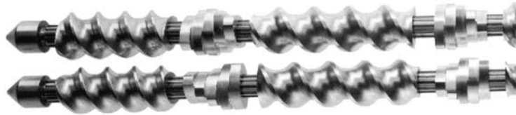
■ Figure 14.8 Configuration of screws in a twin-screw extruder.
