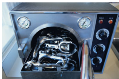
Autoclaves work on the principle of the pressure–temperature relationship of gases, where water in the form of steam is the gas. [Photodisc/Punchstock]
