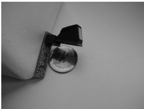
Fig. 5.10 SPREETA TSPR2K11 miniature SPR sensor from Texas Instruments.
