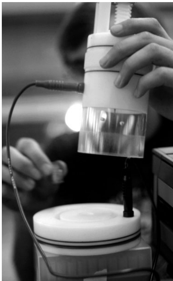
Fig. 16.3. Electroporation of fish eggs. Eggs (15–50) are placed in a DNA solution inside the cuvette and then placed between two electrodes to receive rapid pulses of high voltage.
