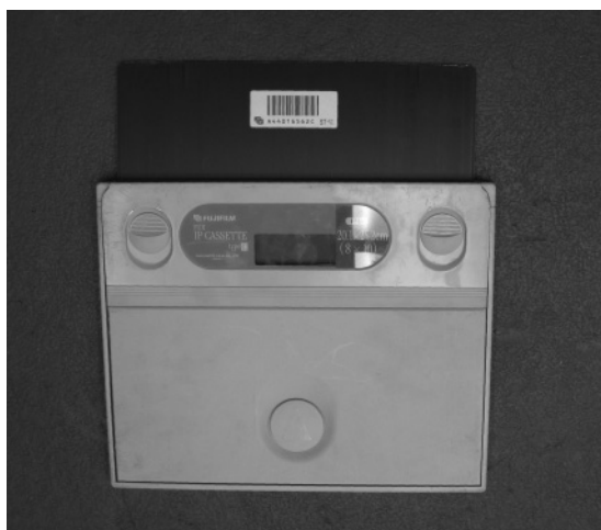
Figure 13.4. Computed radiography detector plate. The image plate has been partially removed from the protective cover.
