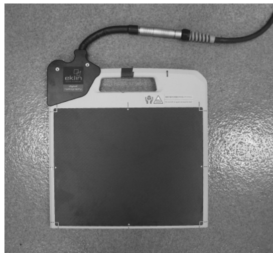
Figure 13.5. Digital radiography detector plate. The fiber-optic cable connected to the computer is seen at the top of the figure.
