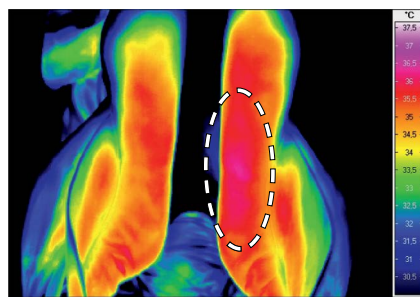
Fig. 4.18. Thermogram of jumping saddle panels taken 30 min after training. The right panel of the saddle puts more pressure on the back (dashed outline).
