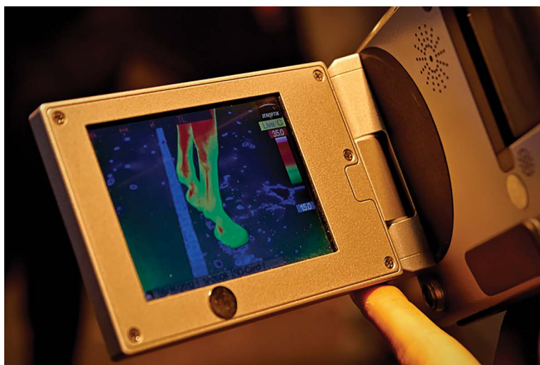
Fig. 1.2. A thermographic camera. The energy distribution of infrared radiation on the horse's distal forelimbs displayed on a thermographic camera screen.
