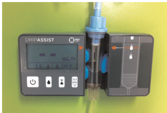
Figure 7.6 A drip counter facilitates monitoring of fluid rate and the total volume administered. Drips of fluid enter the chamber and break a photobeam. This allows the device to count the drip rate and calculate flow rate (mL/hour).
