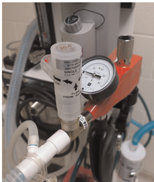
Figure 10.4 A 20 cm H 2 O PEEP valve has been placed in the circuit to prevent development of excessive thoracic pressure when the expiratory port is closed or obstructed. When placed at this location it acts as an anti-PEEP valve. High intra-thoracic pressures are often fatal, and may otherwise develop rapidly when flows appropriate for non rebreathing systems are in use.
