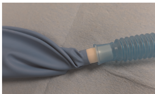
Figure 10.5 The reservoir bag can easily twist at the expiratory port in older T-piece circuits causing occlusion and a rapid increase in pressure. Source: Courtesy of Patrick Burns.
