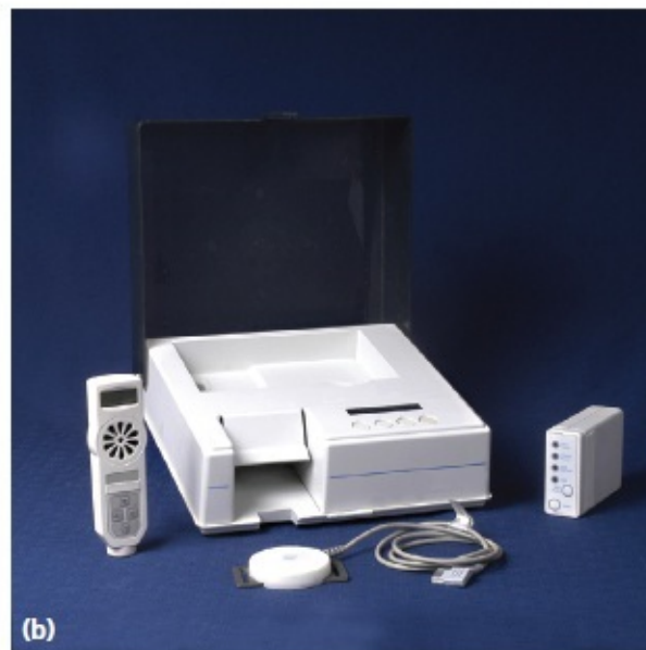
Figure 63.1 (a) A Chihuahua bitch fitted with sensor for a tocodynamometry session. (b) Tocodynamometry unit: modem, recorder and sensor, and hand-held Doppler probe.
