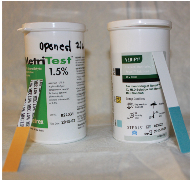
Figure 2.1 Two types of test strips to check HLD concentration. This step should be performed daily and the HLD replaced when strip indicates, regardless of whether the expiry date has been reached.
