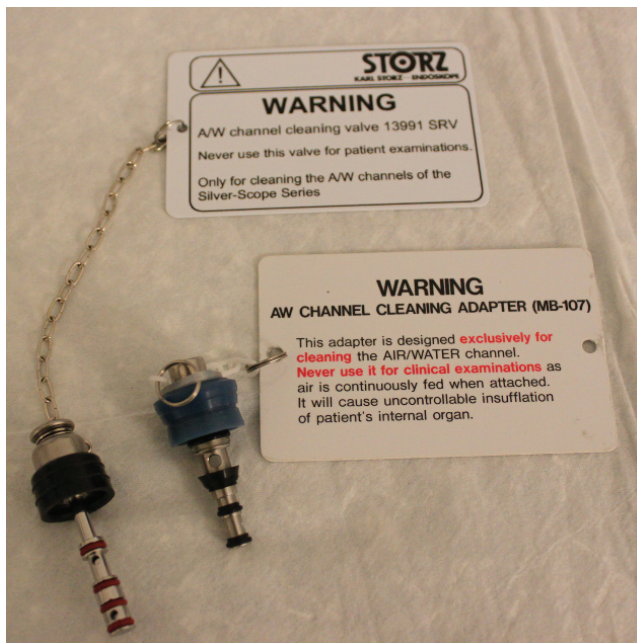
Figure 2.2 Olympus and Storz air/water channel cleaning adapters. Use in place of the air/water valve after the procedure is complete to flush water, then air, through all channels.
