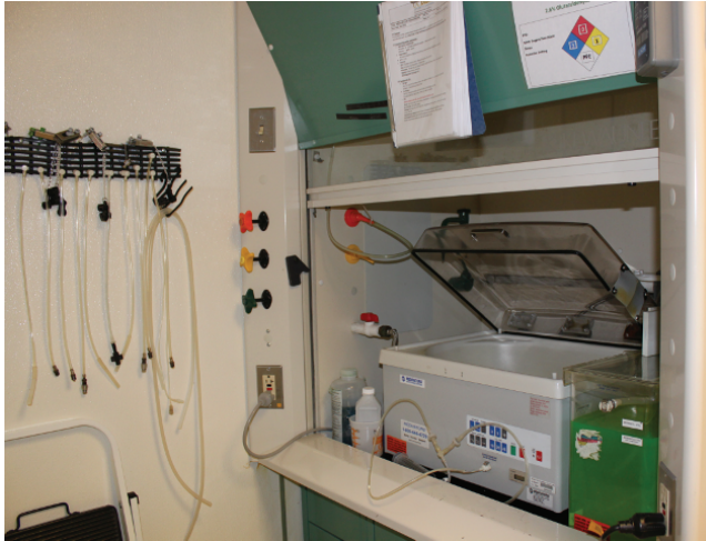
Figure 11.10 An automated endoscope reprocessor in a fume hood. The tank adjacent to the reprocessor houses the high-level disinfection solution. UV and water filters are also connected within the water lines attached to the tub of the reprocessor. Rubber mat pieces attached to the wall neatly hold tubing that connects the endoscope to the reprocessor.
