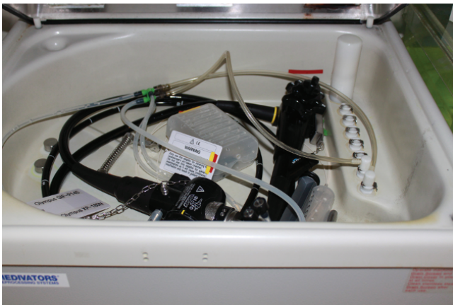
Figure 2.9 An endoscope ready for processing in an automated reprocessor. These types of units save time and reduce exposure to HLDs. To hold small objects such as valves or brushes, a mesh bag or plastic soap holder with perforations may be used.
