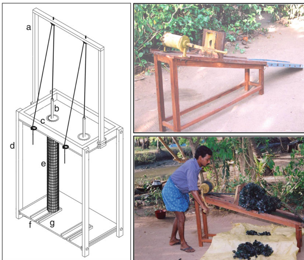
Fig. 3 Details and parts of the mussel seeder (left) (a) top stand, (b) FPS, (c) seed holder, (d) vertical support, (e) PVC pipe, (f) notch for PVC pipe and (g) base plate. Right panel shows the parts of the mussel declumper and its working
