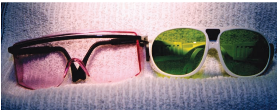
Figure 6-3 Safety glasses for 10,600 nm wavelength (L). Safety glasses for multi-wavelength use (OD 5+ @ 190 nm to 375 nm, OD 5+ @900 nm to 1,070 nm, OD 6+ @ 1,064 nm, OD 6+ @ 10,600 nm (R)).
